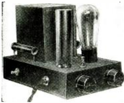
Fig. A. View of the completed "exciter."
