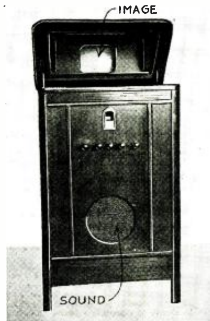
Experimental model of a cathode-ray type of television receiver. Tomorrow's set? (R.C.A.)
