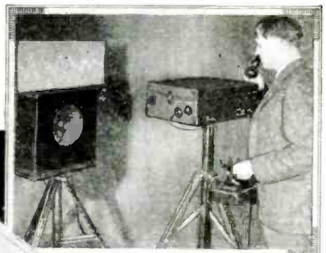
Century of Progress visitors viewed voice wave-forms as pictured at left (waveform—record-recorded), below (oscilloscope unit), and at right (waveform—verbal equivalent of record). A light-beam reflects, from a mirror fastened to a dynamic microphone's diaphragm, to a rotating mirror. (BELL LAB. RECORD)
