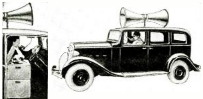
Figs. C and D, below. A French mobile P.A. installation having several novelties. Amplifier and power unit replace a front seat.
