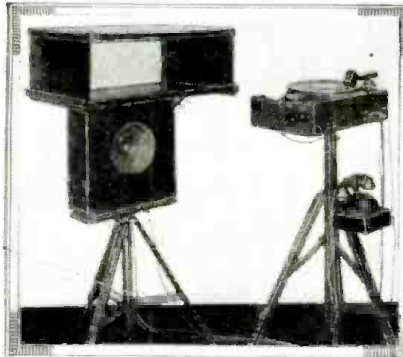
Century of Progress visitors viewed voice wave-forms as pictured at left (waveform—record-recorded), below (oscilloscope unit), and at right (waveform—verbal equivalent of record). A light-beam reflects, from a mirror fastened to a dynamic microphone's diaphragm, to a rotating mirror. (BELL LAB. RECORD)
