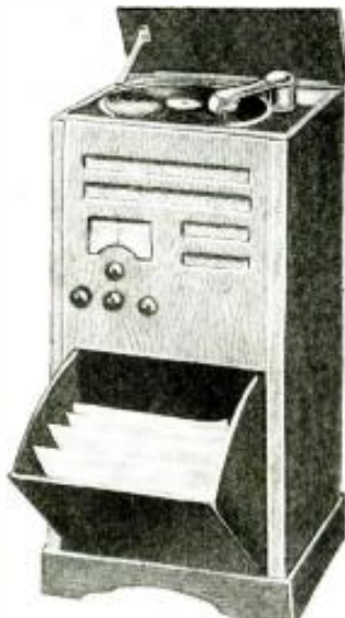
Fig. B. A radio-gram or combined radio and phonograph in a convenient cabinet.
