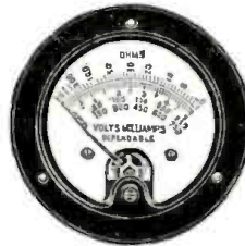
Meter complete with rectifier
