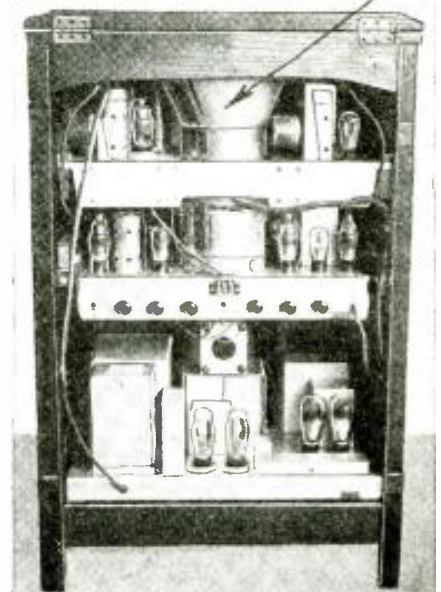
Below, Interior of cathode-ray receiver. (R.C.A.) CATHODE-RAY TUBE MOUNTING
