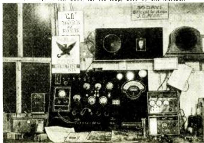
A complete test panel for the shop, built by one member.
