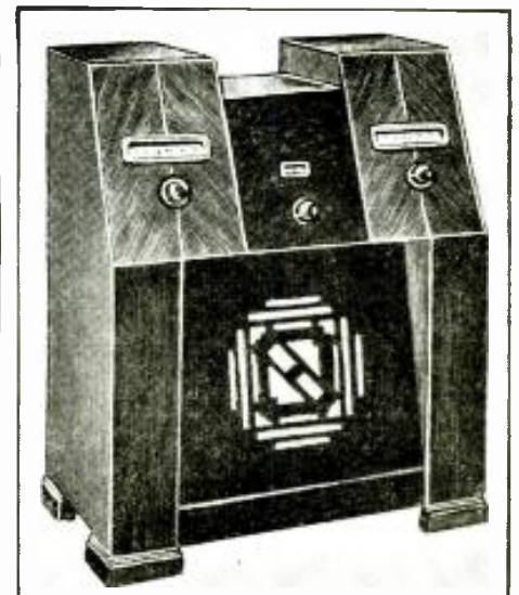
Fig. F, below Three tuning dials are used for the long, intermediate, and short-wave broadcasts.
