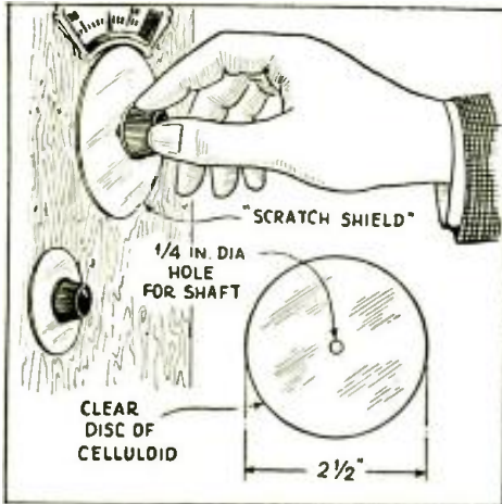
IT IS difficult to grasp the controls of ultra-midget sets without marring the surface finish. The transparent scratch shield illustrated prevents this damage to the cabinet. —E. E. YOUNGKIN
