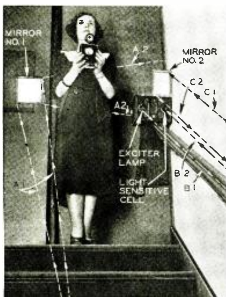
Fig. A Dotted lines A1, B1, C1 indicate light beam courses, and, A2, B2 and C2, reflections.
