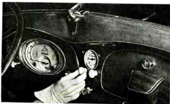
Fig. L, above Standard type installation (Packard), tuning control mounted on steering column. Set mounted behind instrument board.
