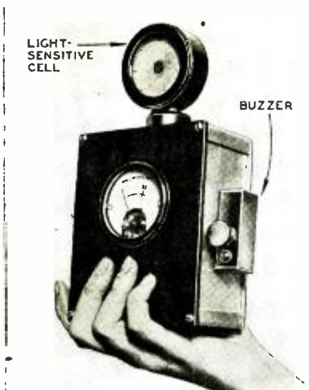
Fig. B The photoelectric guide unit, with its photronic cell on the top and a buzzer on the side.
