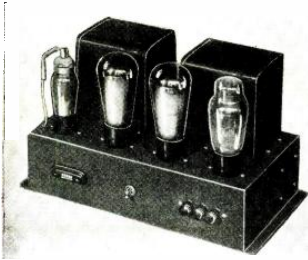
Fig. C, left; Fig. D, above. A 10 W., direct-coupled power amplifier with nearly flat response (left). A 28 W., direct-coupled power amplifier having fine output quality (above).
