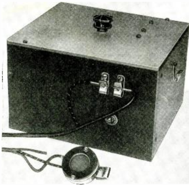
Fig. A Exterior view of the oscillator unit at the "sending" end of the inter-phone.
