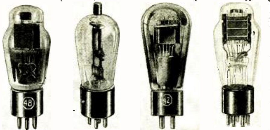
The figure numbers from left to right are A, B, C, and D. Fig. A is the 48, D.C. operated output pentode; Fig. B is the new W.E. amplifier tube; Fig. C, the amplifier-modulator tube; and Fig. D, the 59, A.C. operated output pentode.
