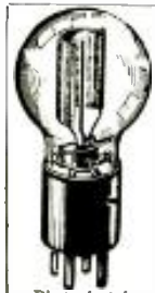
Photoelectric Caesium Type cell.
