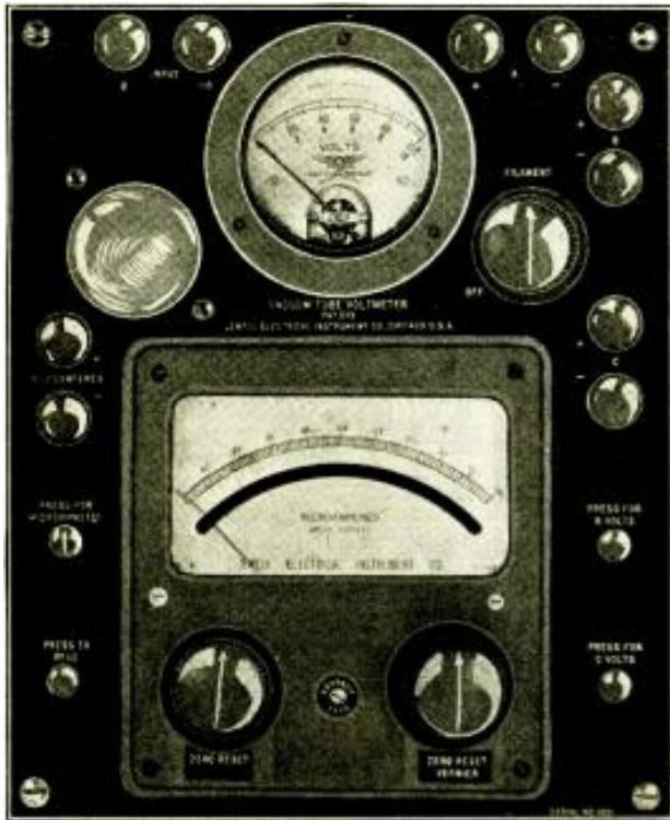
A modern Vacuum Tube Voltmeter (front view).
