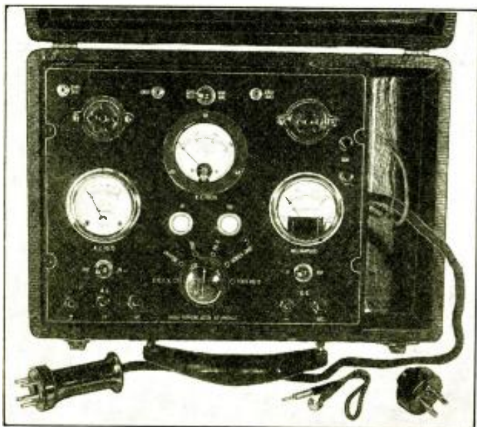
Fig. A (left) Appearance of the R. T. A. set analyzer's panel, seated in the carrying case, with the accessories—plug, adapter, and screen-grid clip (carried with the 3½-volt battery in the compartment at the right). The meters are: upper, Hoyt No. 563 D. C. voltmeter; left, Readrite 0-10-140 A.C. voltmeter; right, Readrite 0-15-150 milli-ammeter.
