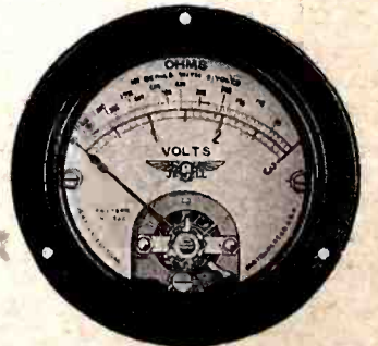
Fig. J A very useful instrument for accurate measurement of values, both of resistors and circuits.
