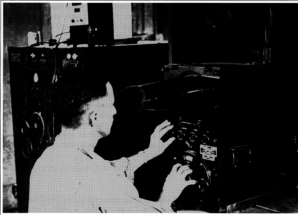
◆ An SCR-270 operator adjusts the oscilloscope controls while viewing the CRT through a glare shield.
