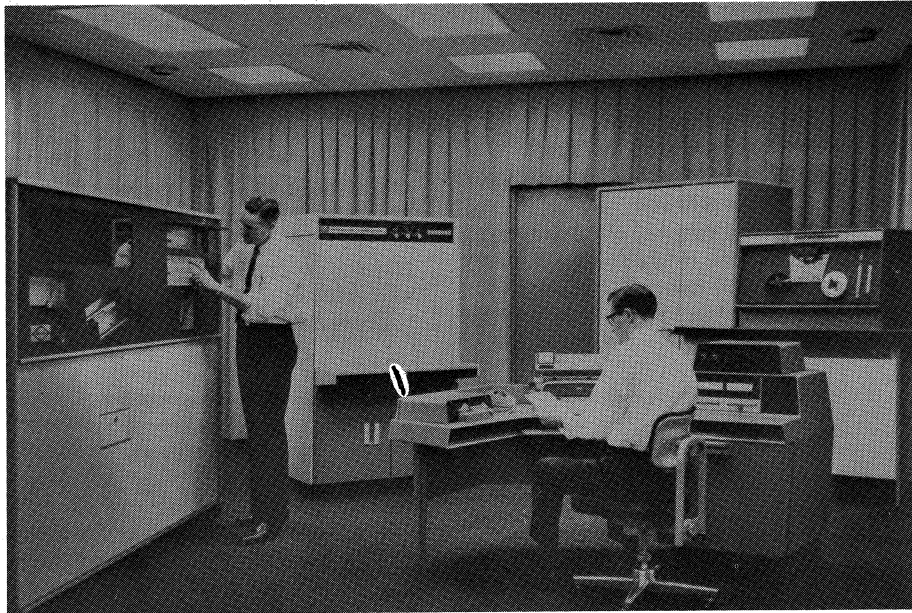
The Farrington Optical Reader is at the left, switching and control center in the foreground, equalizing computer, left rear wall, and Fototronic print-out unit at right rear. This Harris-Intertype system produces finished copy for offset printing directly from typewritten manuscript automatically.
