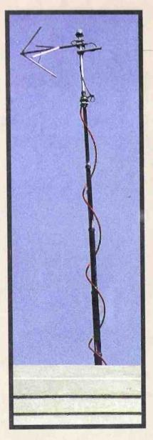
The temporary transmitting antenna for USADR's experimental FM license station. 600 watts, horizontally and vertically polarized with a usable coverage of 6-8 miles. A new antenna and upgrade to 2000 watts is soon to come. (Surprisingly, the test station was received---and confirmed-in RBR's parking lot, a straight-line distance of 34 miles.)
