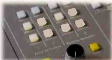
Four special-purpose buses provide automated mix-minus for telephone and remote feeds, each with IFB.
