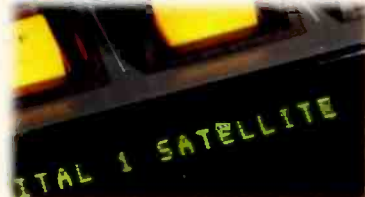
The 10-character display changes when another audio source is assigned, either manually or at a preassigned time.
