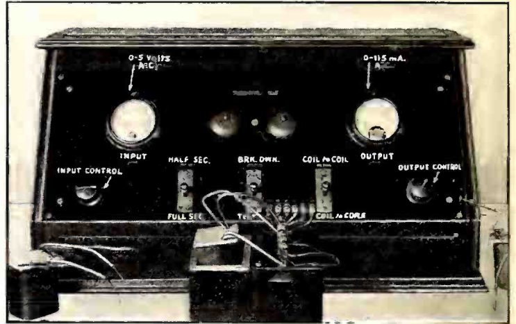
The output transformer test set.
