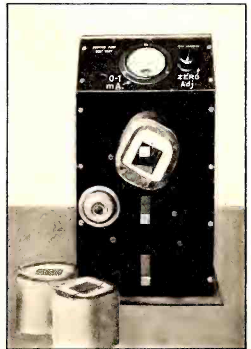
The shorted-turn coil tester.
