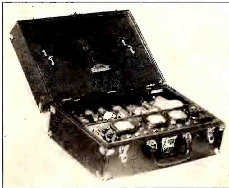
In general service work the Diagnometer is carried in a compact leather case of the type shown above. The case also provides space for accessories and tubes.
