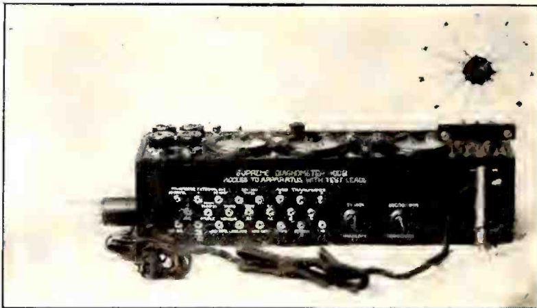
Rear view of Diagonometer showing external pen jacks.
