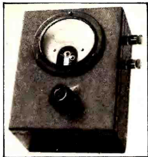
The G.R. 287A ohm-meter will give resistance readings directly without an external battery.
