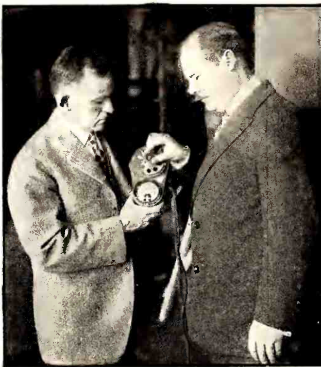
Dr. E. F. W. Alexanderson (right), consulting engineer of the General Electric Company, examining the memory meter which he developed for depth sounding from airplanes. The memory meter intercepts the radio echo and records the altitude for the observation of the pilot. With Dr. Alexanderson in the picture is his assistant, S. P. Nixdorff.
