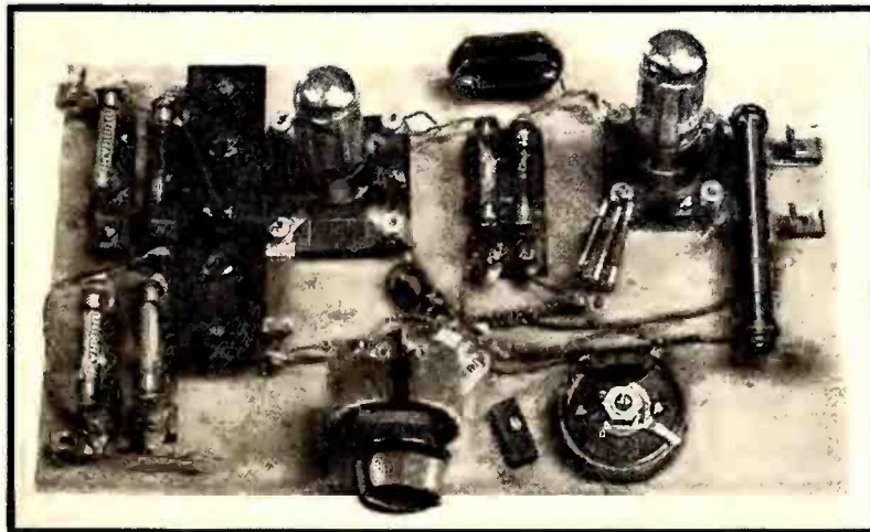
View of the two-tube breadboard-type vacuum-tube voltmeter constructed in the Laboratory.
