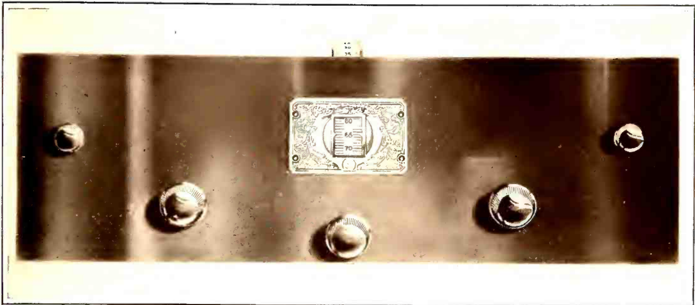
HOW THE COMPLETED TWO-TUBE TUNER LOOKS The five knobs, from left to right, are: "On-Off" switch, trimmer condenser (C 3 ), main tuning control, volume control, regeneration control
