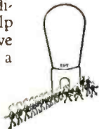
SIGNAL VOLTAGES LEAVING TUBE GREATLY AMPLIFIED BUT SOME RUN AROUND TO ENTRANCE AND CROWD IN WITH THE LITTLE INCOMING SIGNALS
