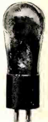
New full-wave gas rectifier tubes. Made under Q. R. S. patent applied for
