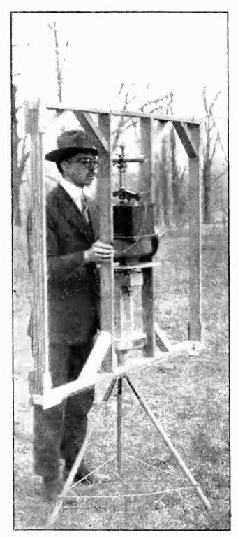
Radio direction finder frame on which telescope is mounted for use in sighting on the radio transmitting station. The scale of degrees is the circular disk just below the hand of the observer
