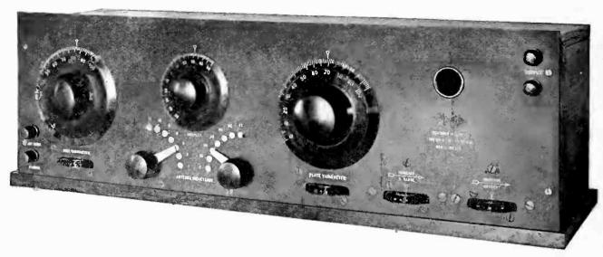
This is a very popular receiving set, covering a wave length range of 150 to 1,000 meters. The set itself is entirely mounted on a single Bakelite supporting panel and is encased by an attractively finished oak box having a hinged cover
