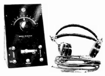
This is a new General Electric crystal receiving set complete with telephone receivers now being featured by the Radio Corporation of America. This little receiver has a wave length range of 180 to 700 meters, made in two steps 180 to 400 and 300 to 700 meters respectively, and tuning is accomplished by a single control to which a pointer is attached which moves over a graduated scale. When the set is not in use, the receivers may be placed inside the metal case by removing the front
