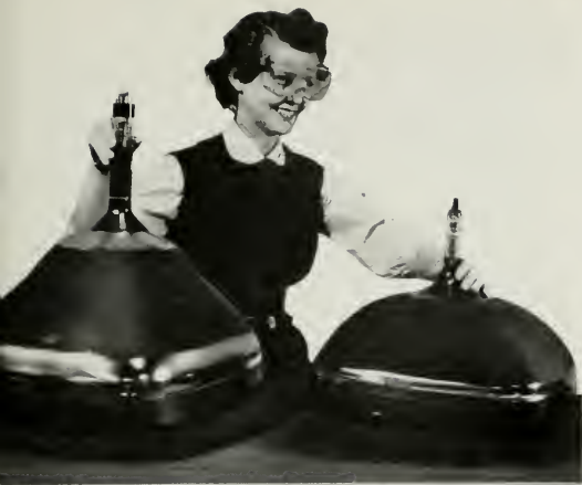
RCA's new 110-degree, 21-inch television picture tube (right) is almost six inches shorter than conventional 90-degree tube (left) and permits more compact styling.
