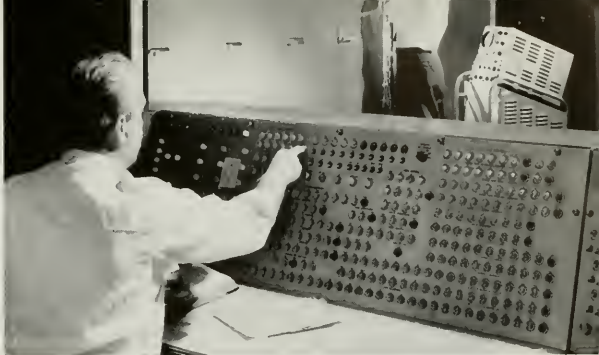
4. The magnetic tape is run through a Sorter, above, which does the electronic equivalent of "paper shuffling"—putting data in the proper sequence.
