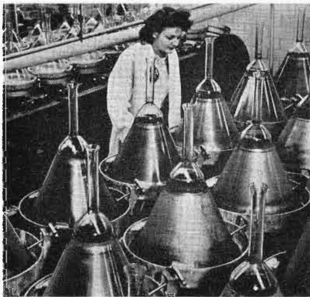
Metal tubes are placed on a crawling conveyor belt to permit the phosphor to settle on the face-plate.
