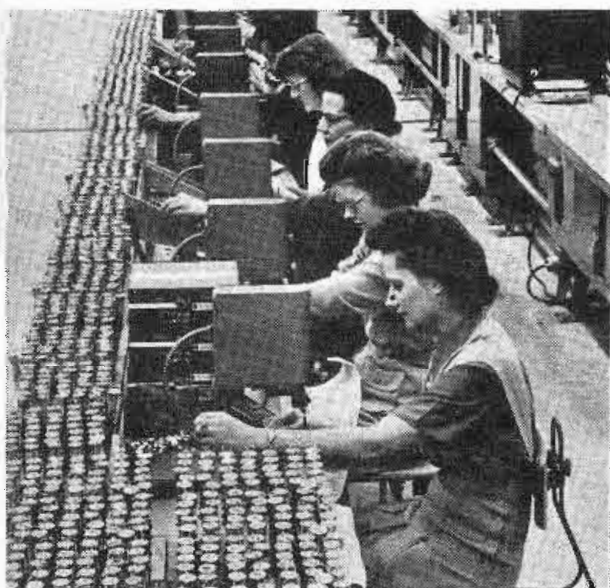
Electron guns are assembled here then microscopically tested to watch-makers' rigid specifications.
