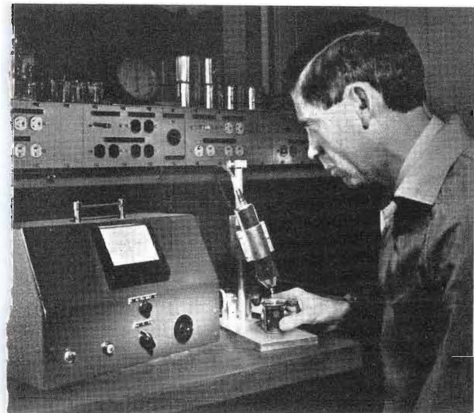
Dr. J. G. Woodward of RCA Laboratories Division demonstrates vibrating plate viscometer.
