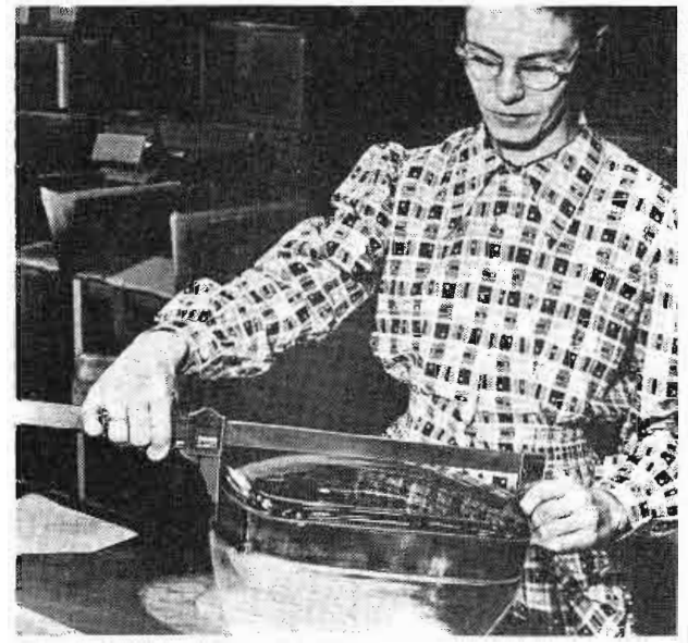
Manufacturing process begins with inspection of all parts comprising the tube, whether glass or metal-shell type.
