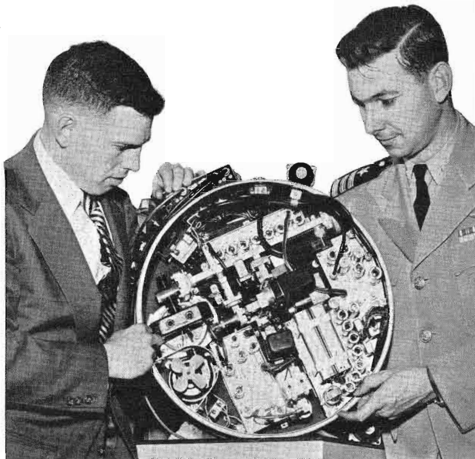
W. B. Kirkpatrick, manager of RCA Victor's Government Radar Unit, and Commander M. A. Mason, head of the Navy Bureau of Aeronautics Radar Section, examine transmitter-receiver unit of new radar.
