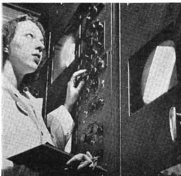
Final tests are made to insure that the tube will give a well-centered perfectly-focused picture.
