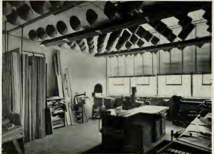
LEFT: TWO CONES CLAMPED TOGETHER AT THEIR OUTER EDGES FORM ONE SILENCING UNIT. BELOW: INSTALLATION OF "CONES OF SILENCE" IN THIS CARPENTER SHOP REDUCED NOISE BY SIXTY PERCENT.
