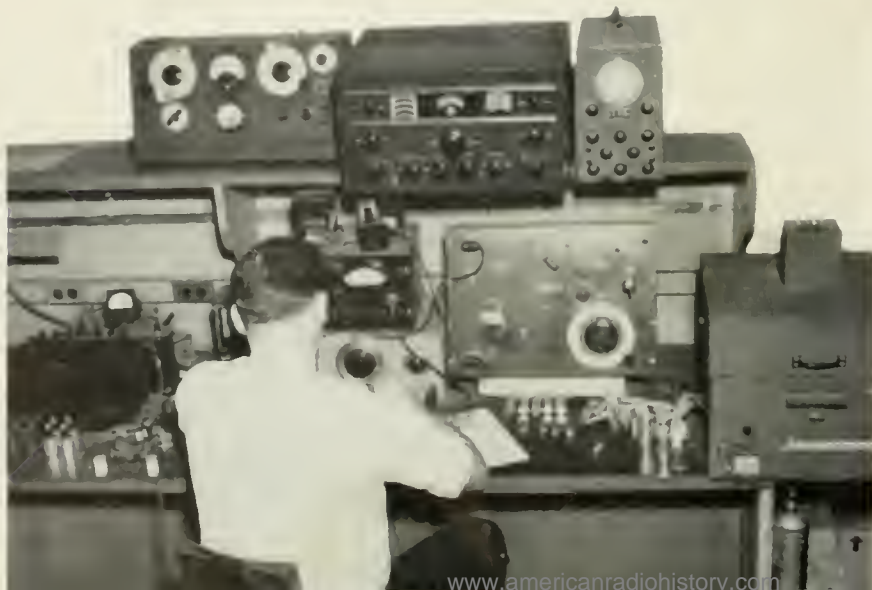
THESE INSTRUMENTS ARE USED TO TEST THE WIDE VARIETY OF CONDENSERS NEEDED IN RADIO AND TELEVISION APPARATUS.
