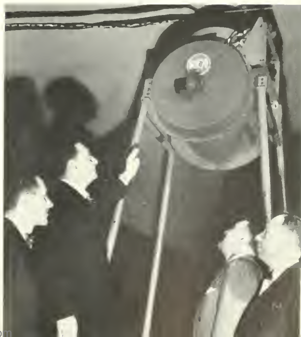
THEATRE-SIZE TELEVISION IMAGES, 15 BY 20 FEET, CAN BE PROJECTED BY THIS TYPE OF EQUIPMENT.
