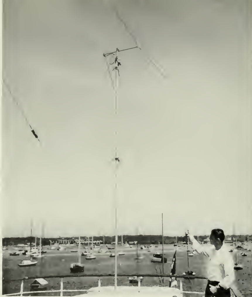
ANTENNA ERECTED ON THE STERN OF THE "SOUTHERN SEAS" CAN BE ROTATED TO ITS BEST RECEIVING POSITION FROM A MOTOR CONTROL BOX ATOP THE TELEVISION RECEIVER IN THE CABIN.
