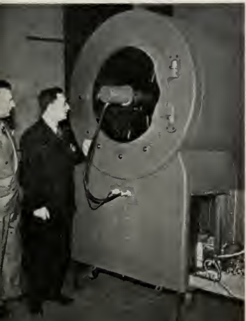
THE AUTHOR AND BARTON KREUZER, MANAGER OF RCA THEATRE AND RECORDING EQUIPMENT, EXAMINE A TELEVISION PROJECTOR GIVING A 15 BY 20-FOOT SCREEN IMAGE.
