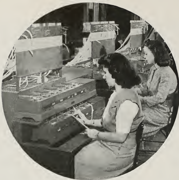
TELETYPE TAPES CONTAINING RADIO-TELEGRAPH MESSAGES FROM FOREIGN POINTS ARE FED INTO THESE MACHINES WHICH AUTOMATICALLY TRANSMIT THE MESSAGES OVER LAND LINES TO THEIR DESTINATIONS IN THIS COUNTRY.
