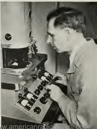
FOUR STEPS IN THE ANALYSIS OF A CHOCOLATE SAMPLE BY ELECTRON MICROSCOPE. AFTER CHIPPING THE CHOCOLATE (LEFT), THE SPECIMEN IS PLACED IN THE VIEWING CHAMBER OF THE ELECTRON MICROSCOPE (BELOW AT LEFT), THEN THE CONTROLS ARE ADJUSTED FOR DESIRED MAGNIFICATION UNTIL THE IMAGE APPEARS AS SHOWN AT THE EXTREME RIGHT.
