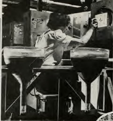
MAKING FINAL TESTS ON 10-INCH KINESCOPES USING A SPECIAL CHART AS A REFERENCE STANDARD.
