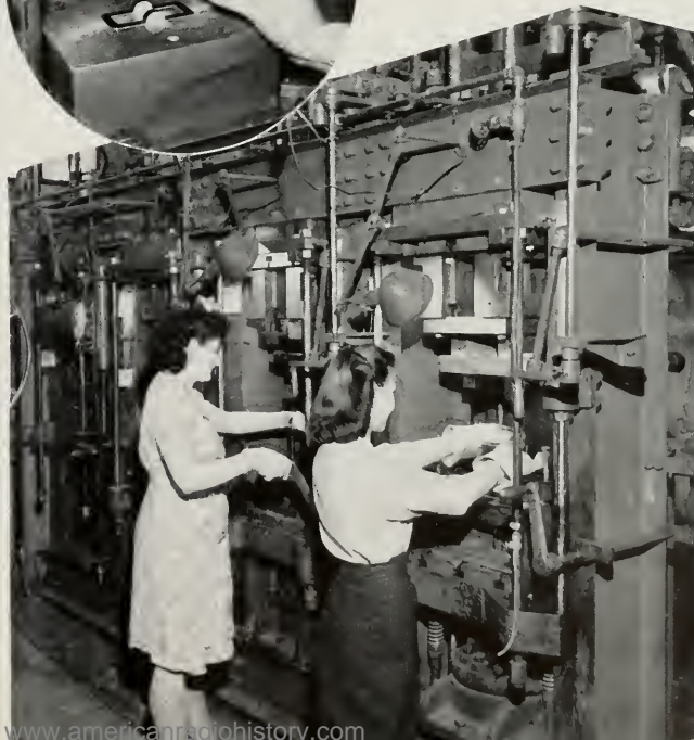
GANGS OF HUGE PRESSES QUICKLY CONVERT PLASTIC MIXTURES INTO POLISHED PARTS FOR RADIO EQUIPMENT.
