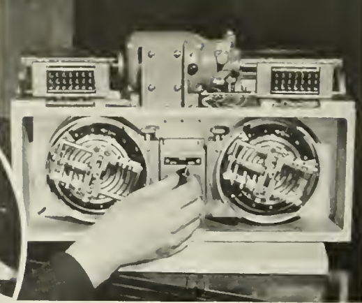
LEFT TO RIGHT: SEVEN-UNIT PRINTER AND PERFORATOR KEYBOARD USED WITH RCAC EIGHT-CHANNEL MULTIPLEX SYSTEM; MULTIPLEX DISTRIBUTOR WHICH ACCOMPLISHES MESSAGE SPEED OF 488 WORDS PER MINUTE; COW-BELL IN CENTER OF FRAME WARNS WHEN AN ERROR OCCURS IN TRANSMISSION.
