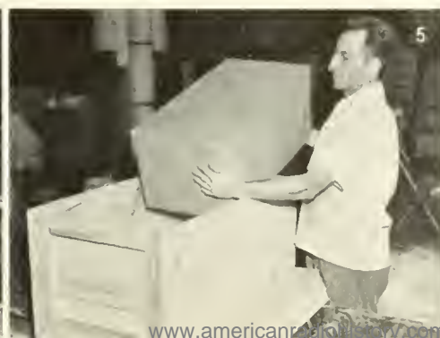
OVER THE FIRST; 4—OVER ALL GOES A SECOND WATER-PROOF ENVELOPE, AND 5—THE COMPLETE PACKAGE, NOW MULTI-PROOFED AGAINST THE RUINOUS EFFECTS OF TROPICAL FUNGUS AND CONTINUOUSLY HIGH HUMIDITY, IS PLACED IN A CRATE FOR SHIPMENT TO SOME DISTANT WAR FRONT.
