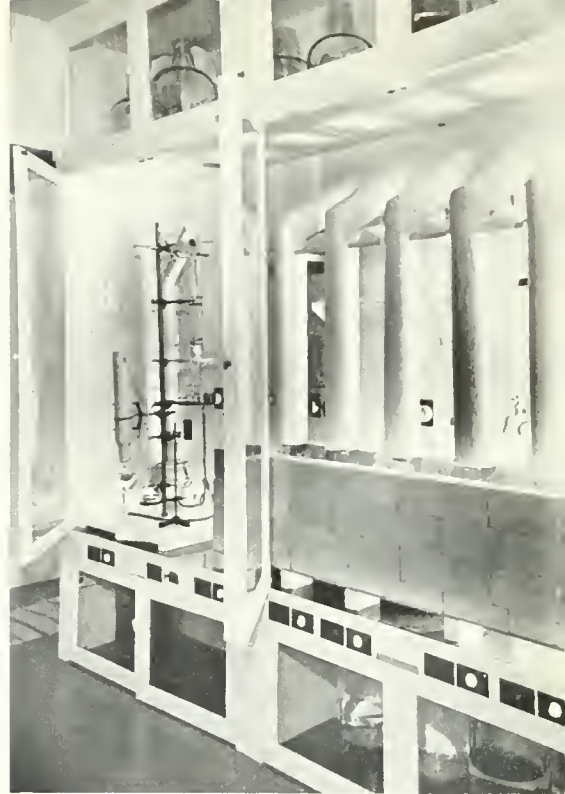
TWO QUARTZ AND FIVE PYREX ELECTRONICALLY-CONTROLLED STILLS FURNISH QUADRUPLY DISTILLED WATER AND ACIDS —THE "LIFEBLOOD" OF LABORATORY OPERATIONS.
