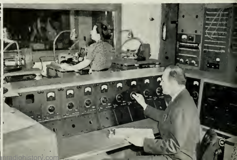
A RECORDING MASTER CONTROL DESK REGULATES THE OPERATION OF THE RCA RECORDING LATHES.
