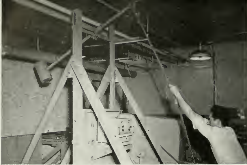
COMMUNICATION EQUIPMENT IS SUBJECTED TO THE POUNDING OF A SLEDGE HAMMER (ABOVE), SIMULATING GUN RECOIL. IN THE "TUMBLER" TEST (BELOW), A ROTATING BOX IN WHICH RADIO AND SOUND UNITS MAY BE DROPPED 1,000 TIMES, IS USED.
