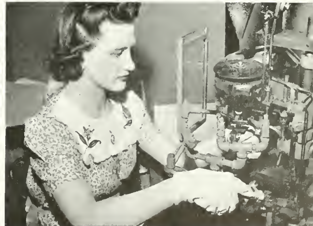
"SUBMERGED" WAS MARKED ON THIS BATTLE-DAMAGED COMMUNICATIONS EQUIPMENT (ABOVE) SENT TO RCA VICTOR FOR RECLAMATION. SEALING TOGETHER PARTS OF MINIATURE TUBES (BELOW) IS ONE OF MANY STEPS IN MANUFACTURING AT RCA VICTOR IN HARRISON, N. J.
