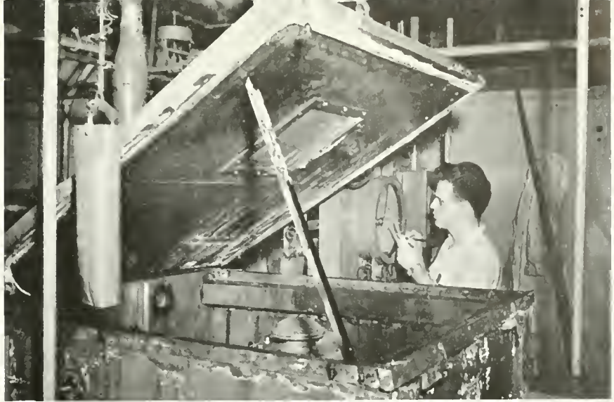
SALT SPRAY AND ULTRA-VIOLET RAYS PLAY ON NAVY COMMUNICATIONS EQUIPMENT IN THIS TEST (ABOVE) TO DETERMINE ITS CORROSION RESISTANCE. EQUIPMENT IS CHECKED FOR WATER-TIGHTNESS AFTER IT HAS BEEN SUBMERGED IN A LARGE TANK (BELOW) FOR A NUMBER OF HOURS.
