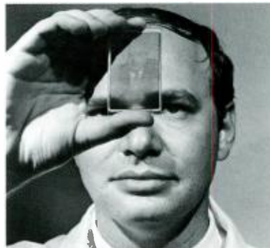
Portrait image on a photochromic surface is instantly obtained by exposing the material to blue light through a photographic negative. It can be erased by yellow light.
