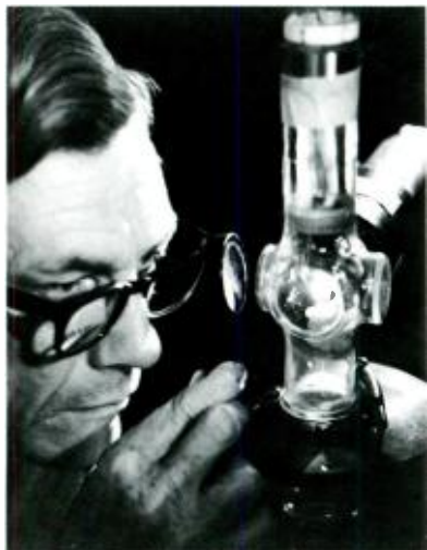
Experimental display unit, made up of hundreds of tiny semiconductor lasers, may one day be able to project color TV pictures on a wall.
