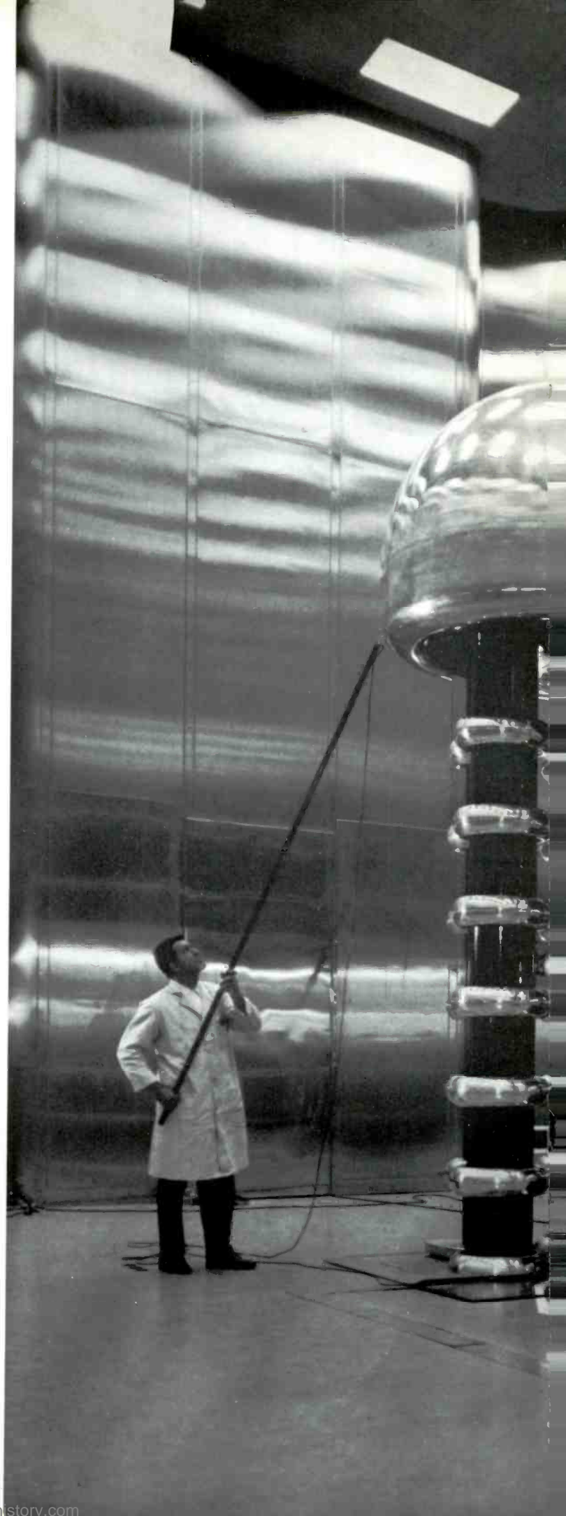
Accelerators for U. S. Steel's electron microscope drive its electron beam at nearly the speed of light.
