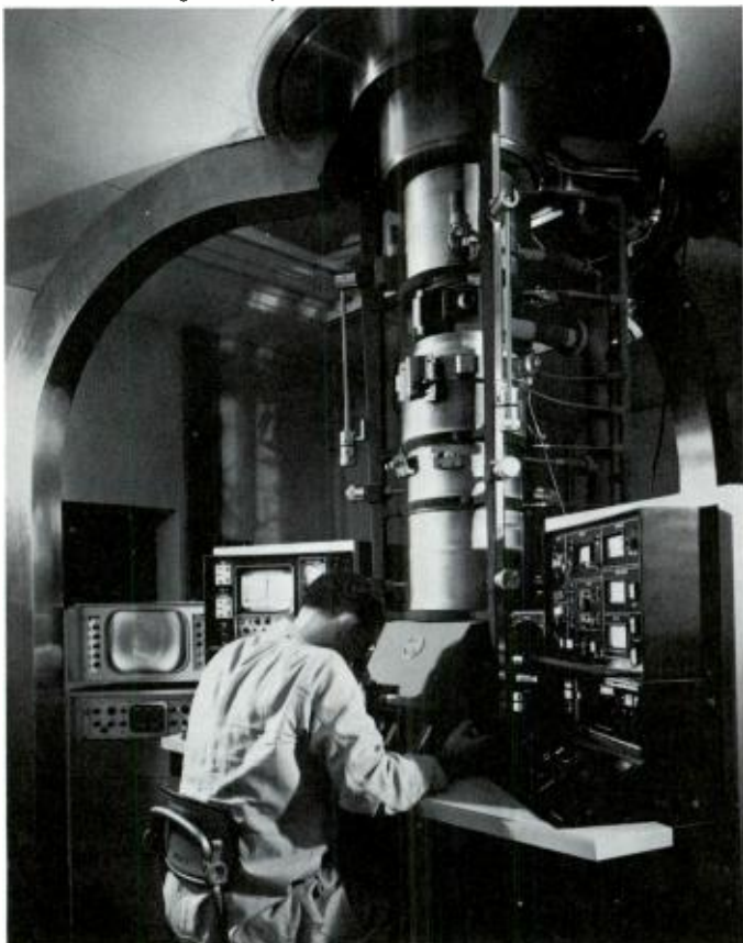
RCA electron microscope at the U. S. Steel research laboratory in Monroeville, Pa., is used for metallurgical analysis.
