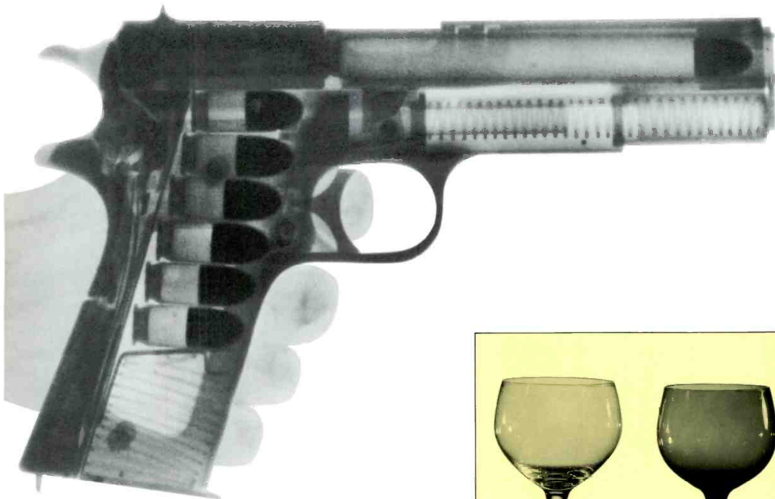
A “flash X-ray” photograph of a pistol at the moment of firing.
