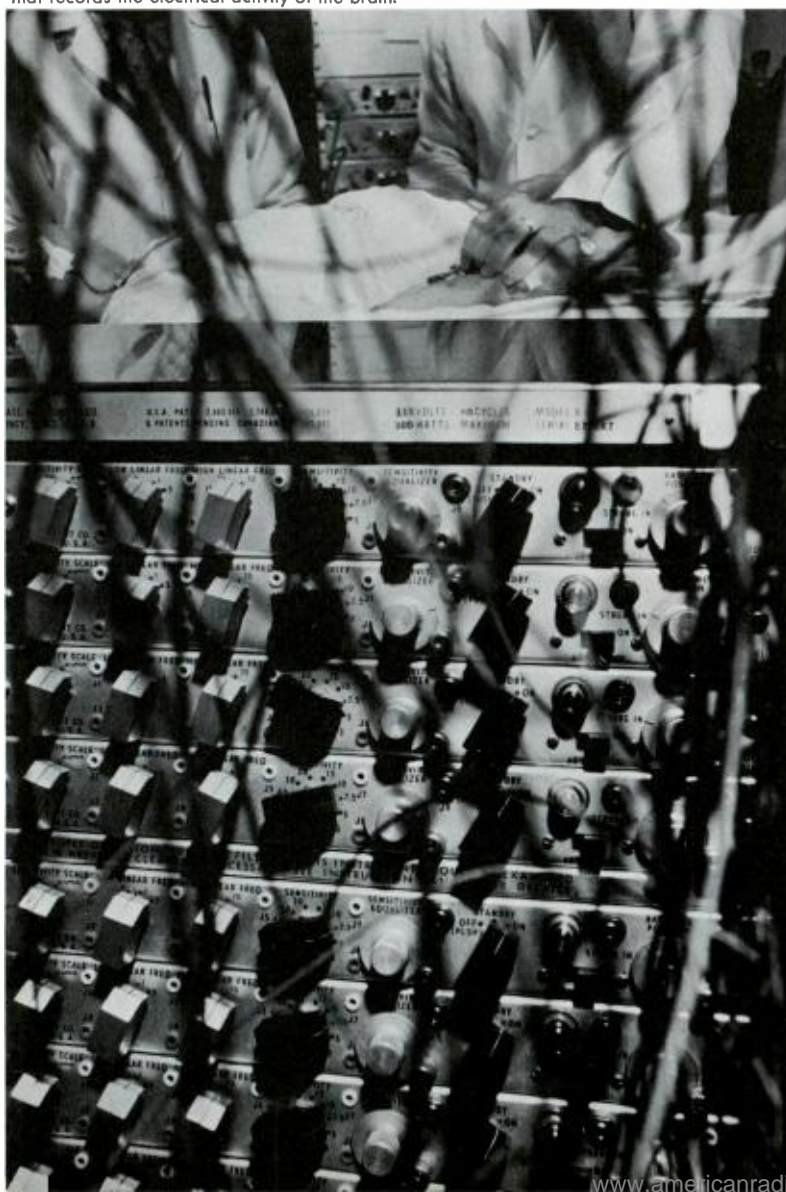
A patient is wired to an electroencephalograph, an instrument that records the electrical activity of the brain.
