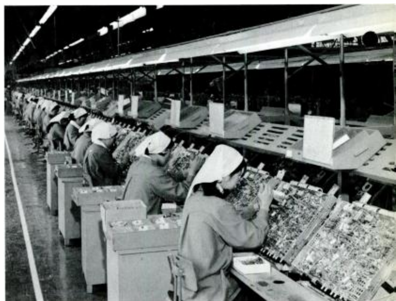
Workers assemble color television chassis at the Tokyo Shibaura Electric Company, the largest manufacturer of color sets in Japan.
