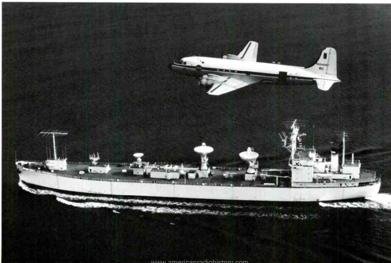
A NASA instrumentation aircraft checks out the Vanguard , one of the five tracking ships outfitted for the Apollo program.
