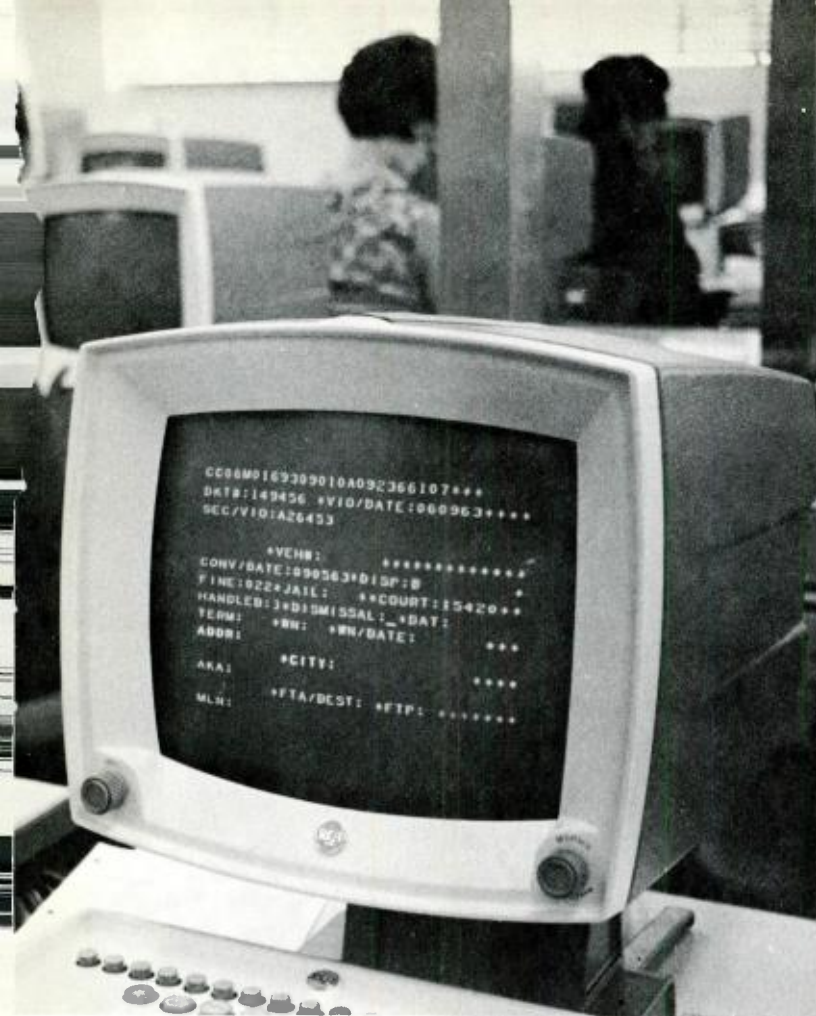
Motor vehicle records are displayed directly from a data bank onto the screen of a video display device. The system is part of the California Department of Motor Vehicles huge computer-communications network.
