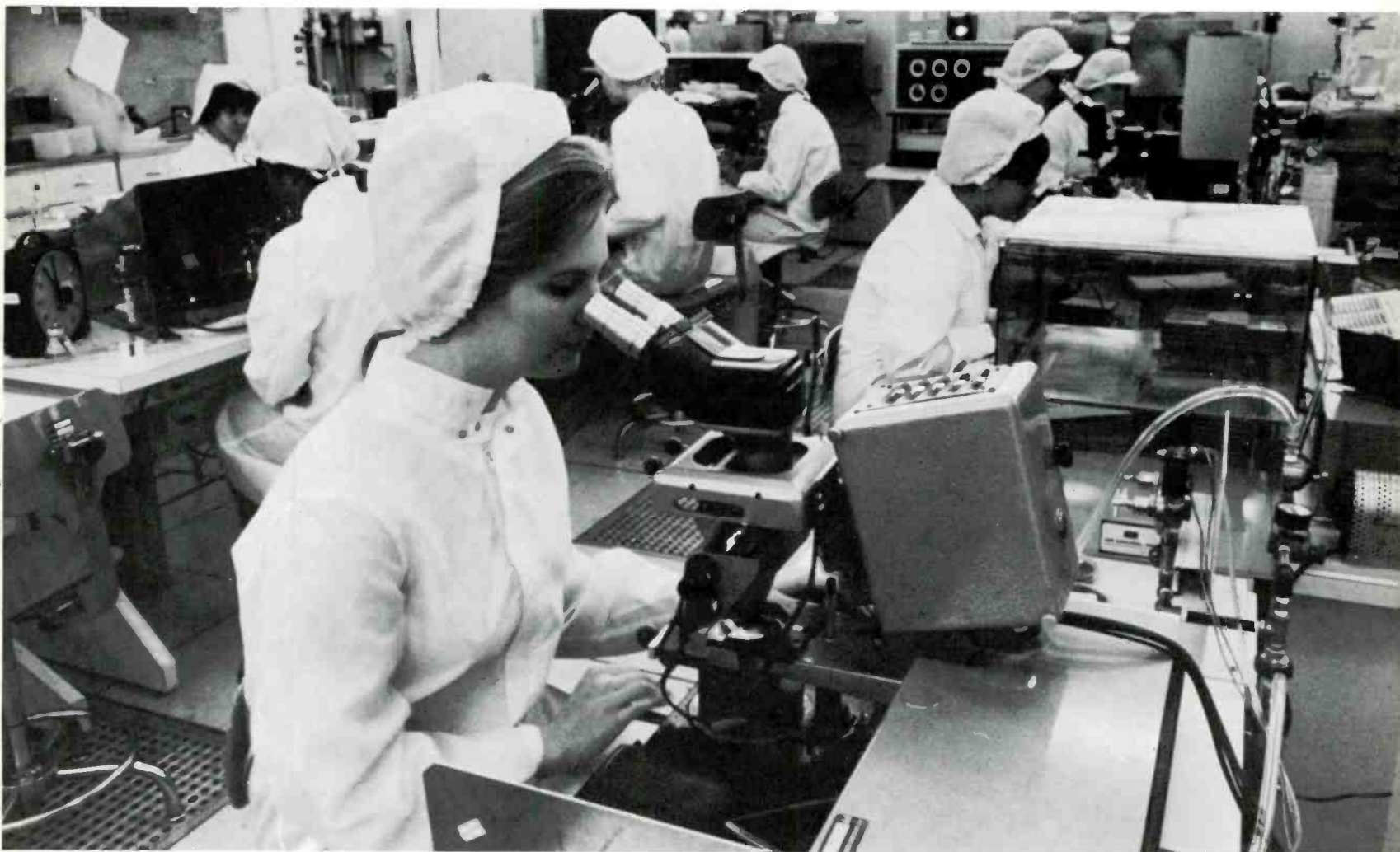
Microscopes are used to inspect a wafer of silicon on which have been etched a number of tiny integrated circuits.
