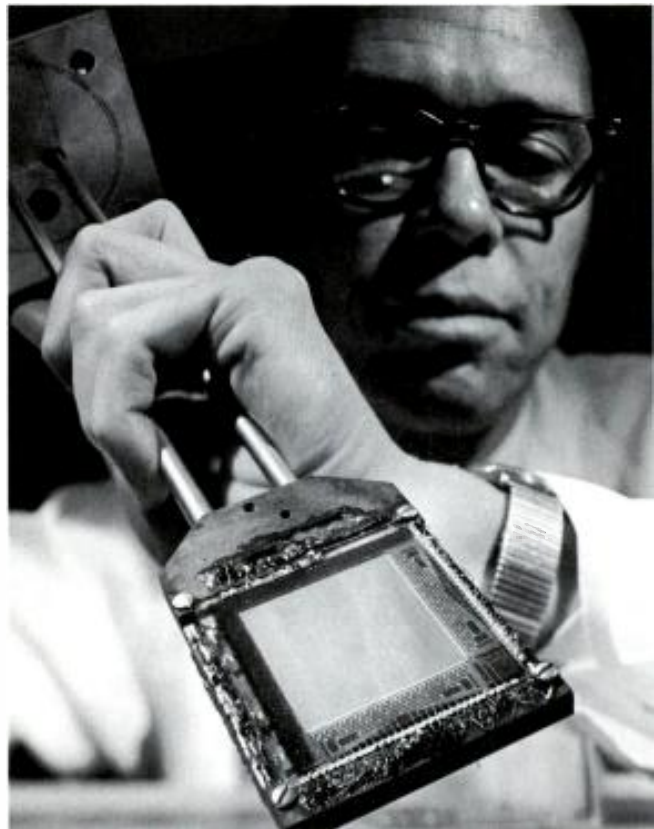
Operating in liquid helium at a temperature close to absolute zero, this revolutionary computer memory takes advantage of the phenomenon of superconductivity to store 16,384 bits of information.
