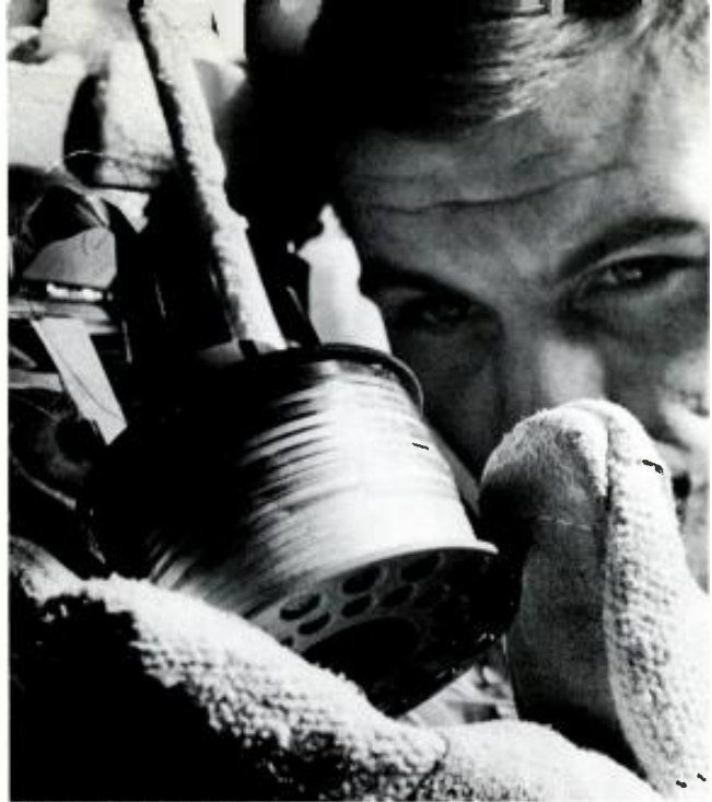
Superconductive magnets like the above can generate magnetic fields that can exert 12 tons of pressure per square inch.
