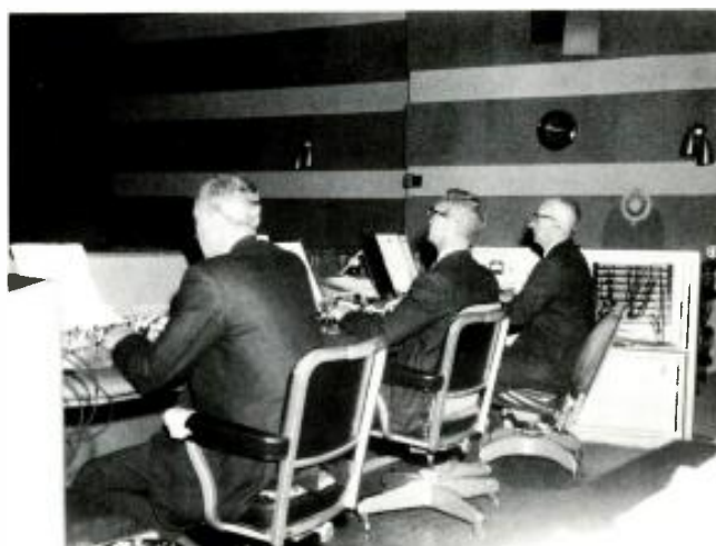
Experts at mixing console can blend as many as fourteen separate sound tracks into one composite track.
