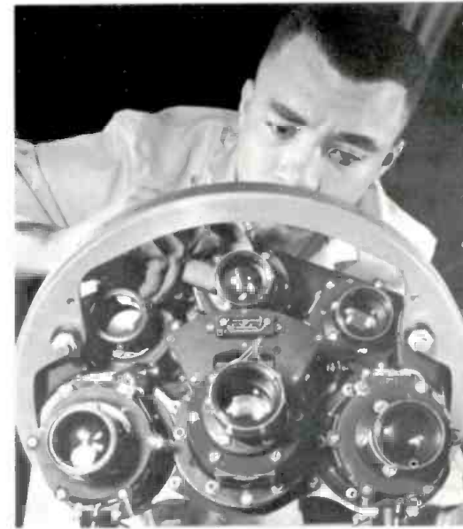
Six TV cameras of the Ranger VII television system, designed and built by RCA, returned first closeup photos of the lunar surface.
