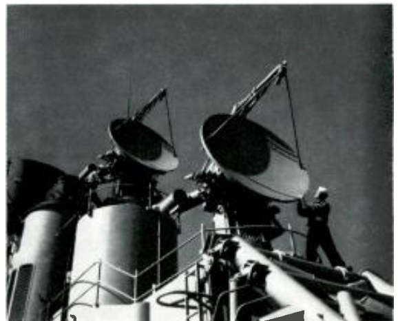
These fire control radars (above) on guided missile destroyers help guide Tartar missiles despite enemy evasive tactics or jamming.
