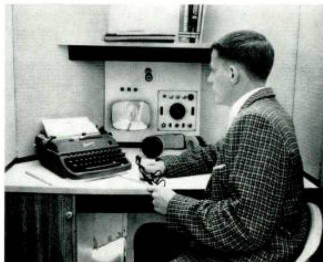
Interior of carrel shows unique features, including soundproof panels, television screen, selective dialing system, and earphones for audio instruction.
