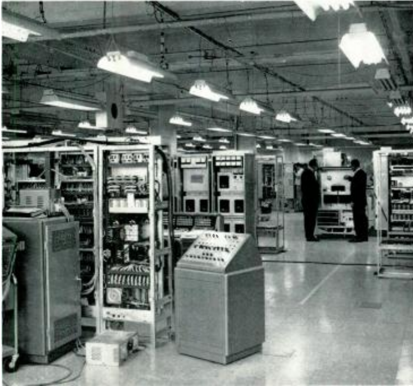
Units of a DATACOM switching center undergo final testing at RCA's Camden, N. J., manufacturing plant. An entirely new concept in communications handling, DATACOM/AUTODIN is now installed in key Air Force centers.
