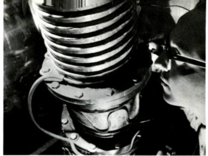
Producing temperatures that melt iron and pressures that equal an ocean depth of 2,000 feet, this autoclave is creating gallium phosphide, a new semiconductor material.
