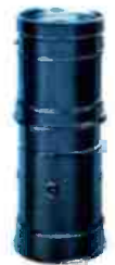
RCA Image Converter Tube amplifies light more than 50 times—then “snaps” a picture in 1/200 millionths of a second.
