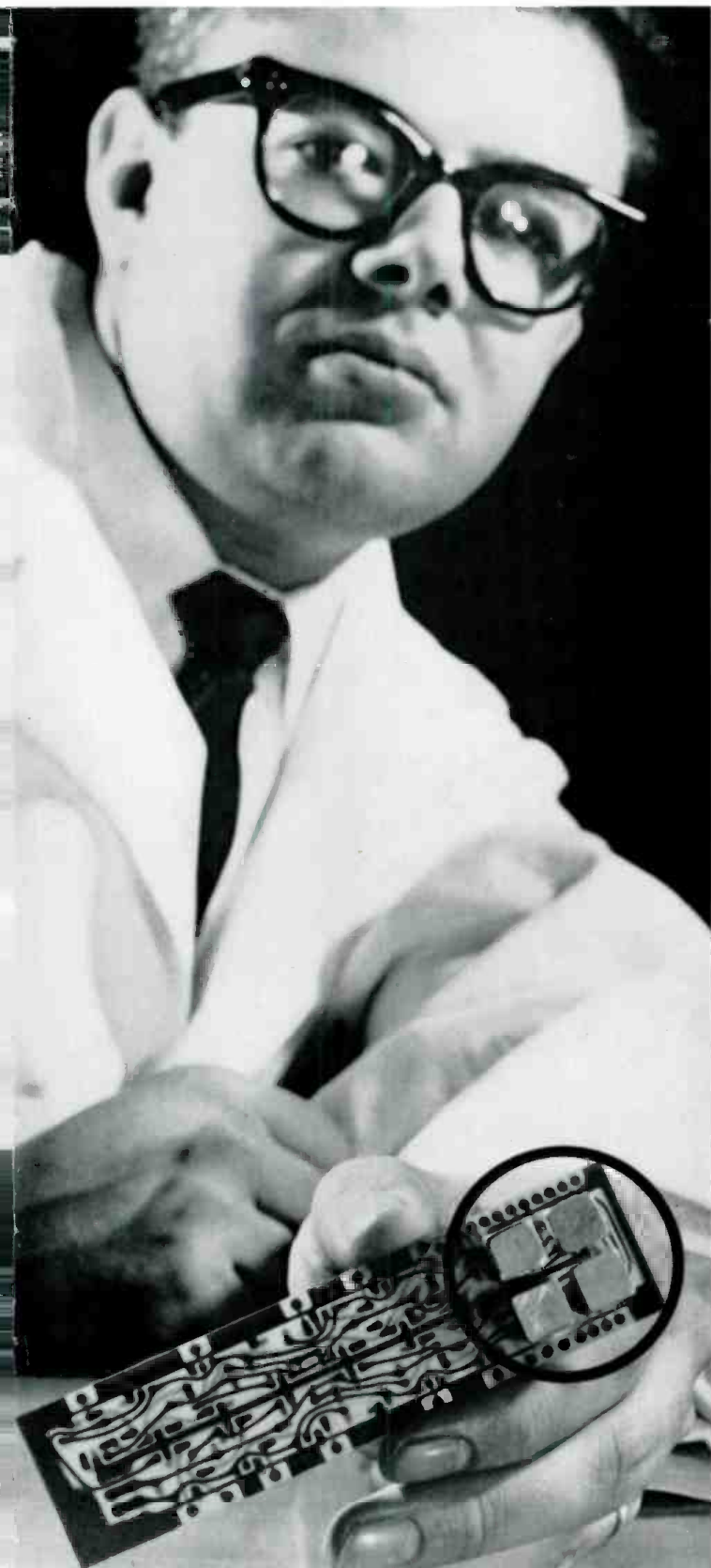
Printed circuit board held by RCA engineer in laboratory contains four micromodules (circled in upper end of board).
