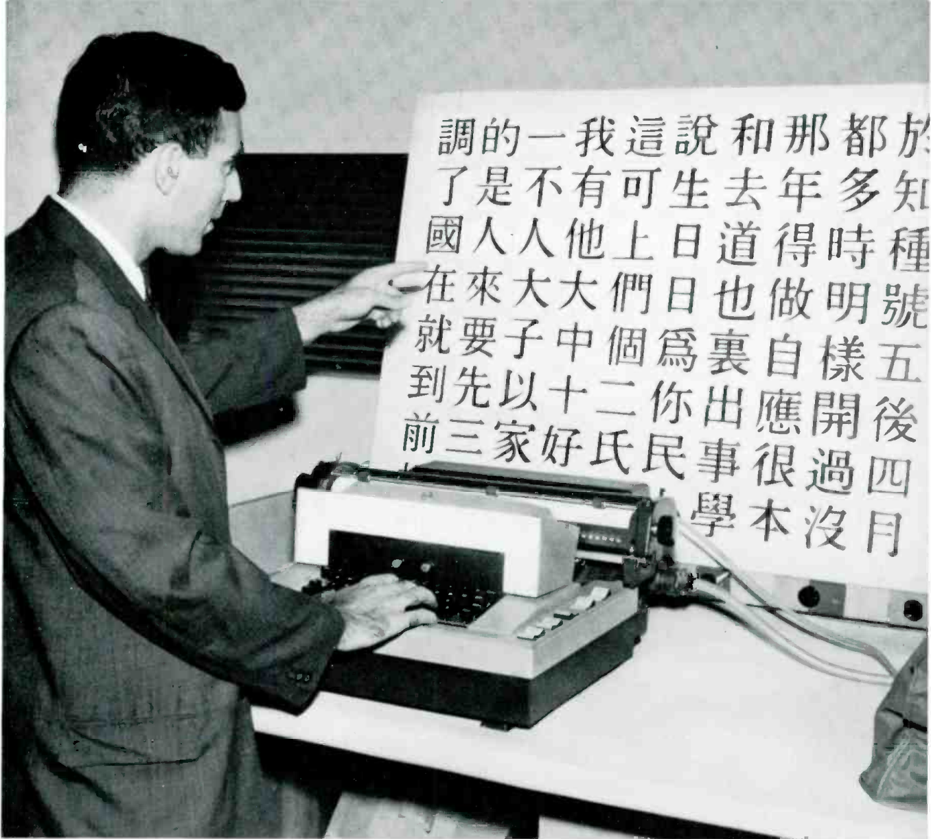
History's first Chinese typesetting machine uses only a 41 symbol keyboard to produce the 10,000 characters of Chinese for printing.
