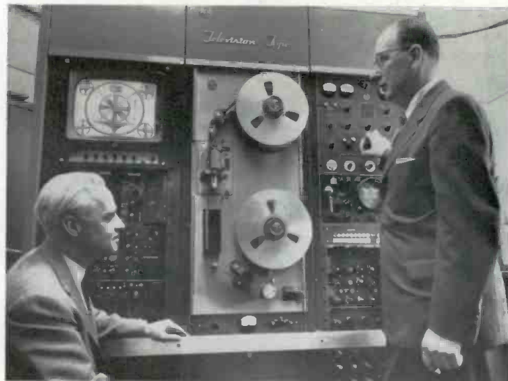
New RCA television tape recorder, with E. C. Tracy and C. H. Colledge, of Broadcast and Television Equipment Division.
