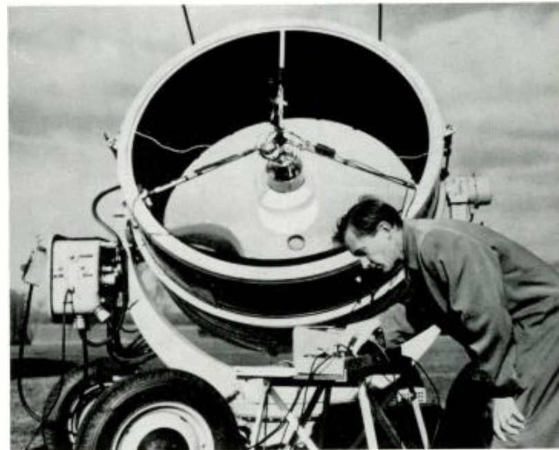
Solar furnace is tested at David Sarnoff Research Center, Princeton.
