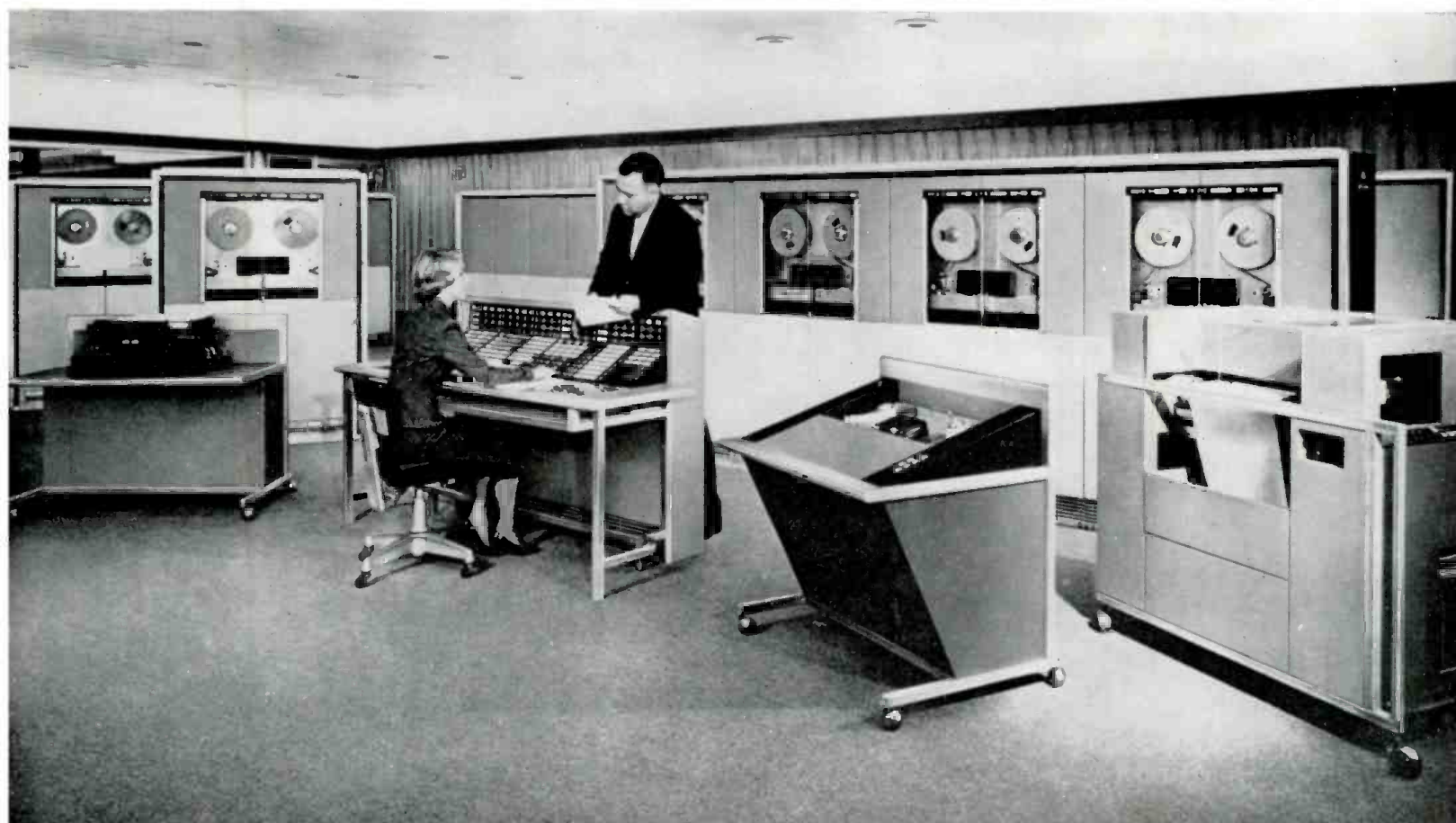
Operator at control console of RCA 501 all-transistor computer receives instructions for handling a data processing assignment.
