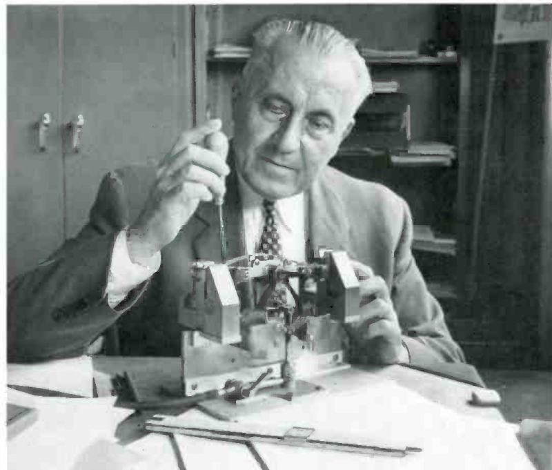
Thermoelectric motor converts heat to electric current at RCA Laboratories.
