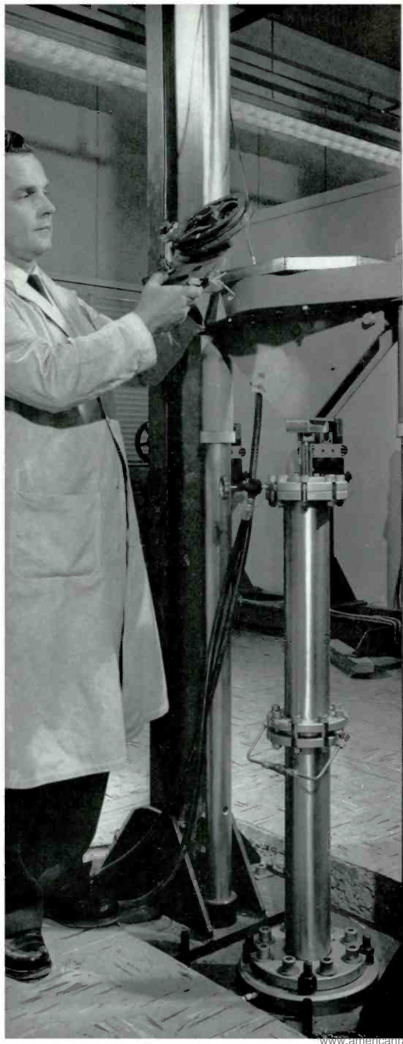
I. G. Harrett of the RCA Astro-Electronic Products Division places a TV tape recorder for a satellite on a special shock tester.
