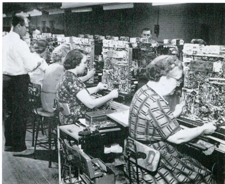
2. Inspectors give completed chassis thorough check before it is moved to final assembly area.
