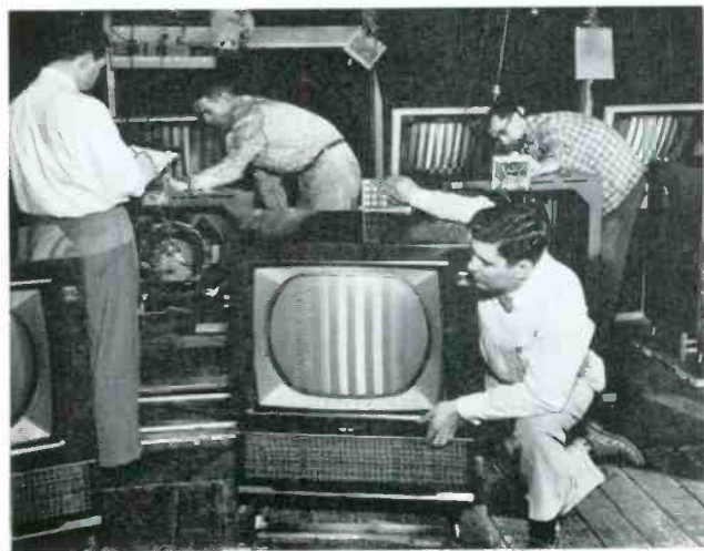
5. Series of mirrors in rear permit inspectors to make adjustments quickly and easily from the rear of the set.
