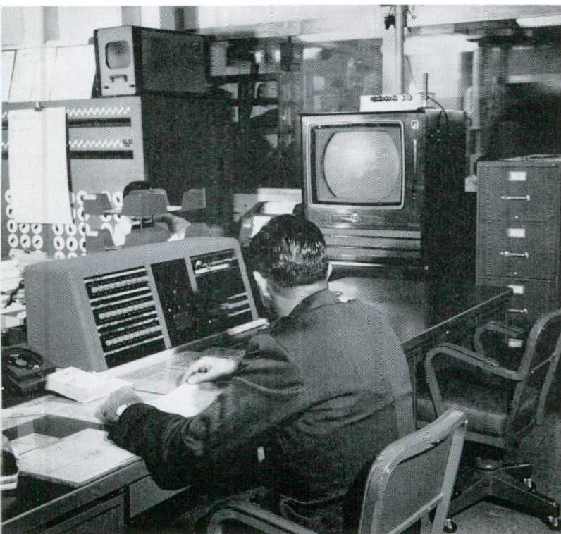
The SAC Controller can see any portion of main operations room without moving from chair. He can reach any SAC base in world through telephone switch console.
