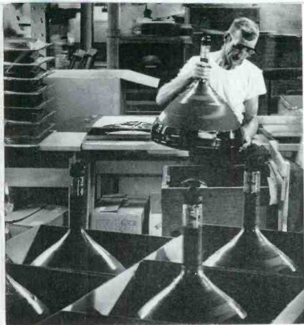
3. RCA tri-color picture tube, heart of a color receiver, is inserted along with kinescope mask—on bench at left.
