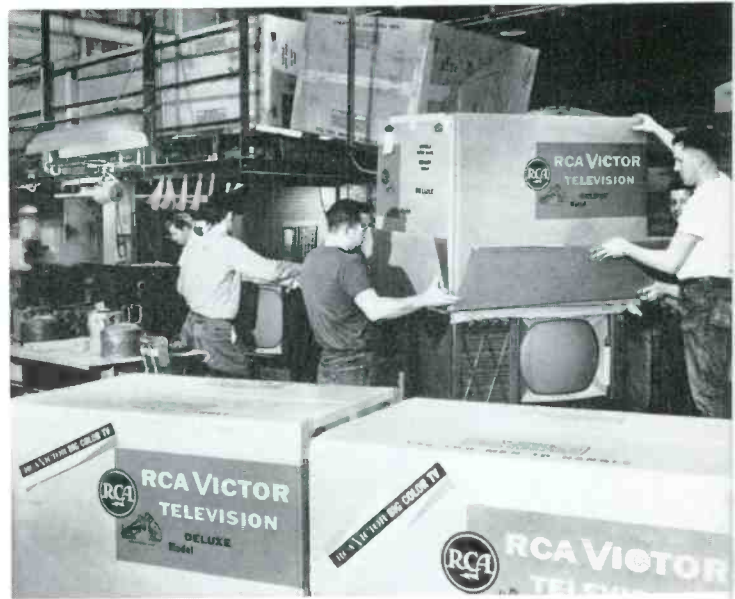
7. Final step is packaging completed set. Empty carton has followed cabinet along assembly line.
