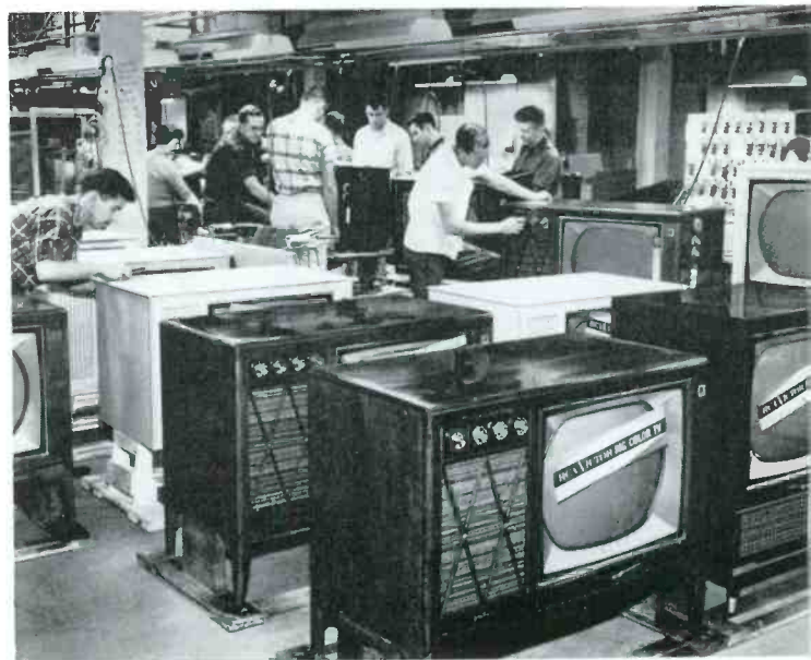
6. Before protective rear cover is installed cabinets are given final check, then sent to packing area.
