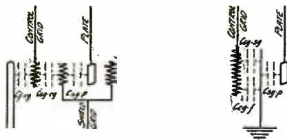
A SCHEMATIC REPRESENTATION OF A SCREENED-GRID VALVE
