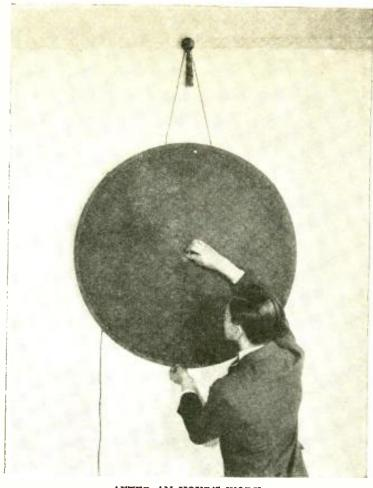
AFTER AN HOUR'S WORK The completed cone is quite distinctive in appearance when hung on the wall by means of the cord. And its tone quality, if the cone is assembled with reasonable care, should be equal to that of the best manufactured reproducers of this type.
