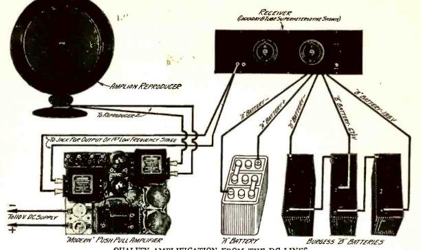
QUALITY AMPLIFICATION FROM THE DC LINES FIGURE 1: The hook-up shown above should bring cheer to those who live in neighborhoods where direct current is employed. The Modern push-pull amplifier, at the lower left, is shown supplying a 371 valve push-pull stage of low-frequency amplification for the Cockaday 8-valve superheterodyne.
