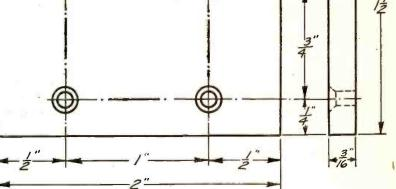
HOW TO DRILL THE PANELS FIGURE 4: The two small panels for the binding posts, 11 and 12, and 13 and 14, should be cut and drilled according to the above layout.
