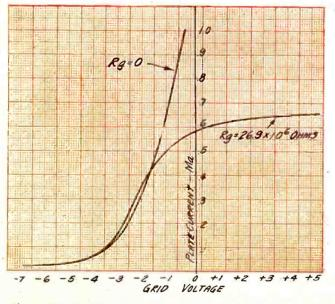
FIGURE 2: A grid-voltage, plate-current characteristic of a vacuum valve, showing how this factor varies with different conditions of grid resistance.
