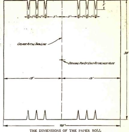
THE DIMENSIONS OF THE PAPER ROLL FIGURE 3: The roll should be cut along the solid lines around the edge and creased along the broken vertical line in the center.
