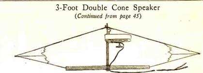
A CROSS-SECTION OF THE COMPLETED UNIT FIGURE 4: In this cul-away diagram of the cone the method of attaching the driving unit is clearly shown.
