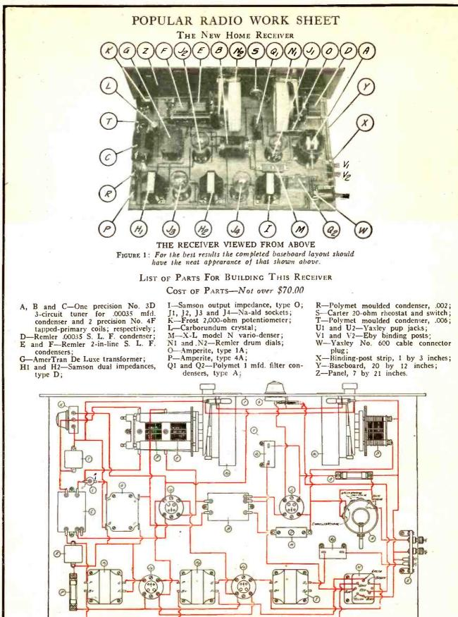
HOW TO WIRE THE RECEIVER FIGURE 2: The instruments are outlined in BLACK; the wiring is all done above the baseboard, and is indicated in RED.
