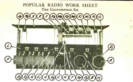
THE LAYOUT OF THE INSTRUMENTS FIGURE 2: Note the individual shields of heavy copper tubing around the high-frequency and detector stages at the right.
