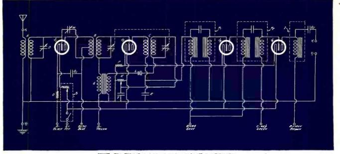
THE CIRCUITS OF THE NEW HOME RECEIVER FIGURE 3: The high-frequency amplifier is at the left in the schematic diagram; the double-impedance-coupled, low-frequency amplifier and output filter at the right. The crystal detector is shown at L, followed by the reflex transformer, G.
