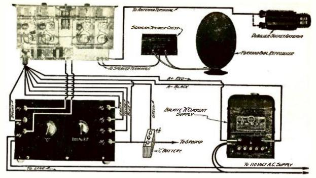
AN EXCELLENT POWER HOOK-UP FOR THE HI-Q FIGURE 1: In the hook-up shown here the Hi-Q receiver is operated entirely from the AC lighting lines, with the exception of the small, semi-permanent "C" battery. The units shown here were found by tests to give excellent results when hooked up as indicated by the heavy black lines.
