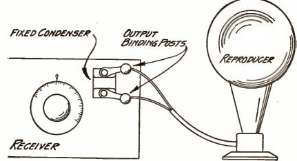
ONE WAY TO BETTER REPRODUCTION FIGURE 5: A small fixed condenser connected across the output binding posts brings out the low notes with great clarity.
