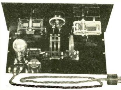
AN INSTRUMENT FOR NEW RADIO DISCOVERIES By plugging this simple unit into any standard broadcast receiver, the radio listener can bring into his receiving range all the absorbing radio traffic that goes on at the short wavelengths-amateur conversations, transatlantic calls and short-wave broadcasts.
