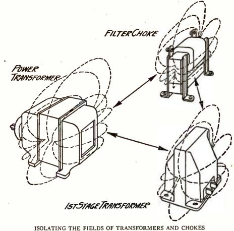
FIGURE 1: Interaction between the magnetic fields of transformers and choke coils is one of the most common sources of hums. In their efforts to get a simple and compact layout, many set builders crowd their instruments, with disastrous results. The spacing shown in this diagram is an example of good spacing of instruments. Notice that the fields, shown in dotted lines, do not interlink, but are separated by distances indicated by the arrows.
