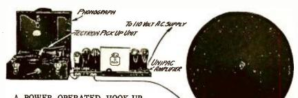
A POWER OPERATED HOOK-UP FIGURE 4: By the use of the LC-28 Unipac amplifier, and suitable reproducer and pick-up units, batteryless reproduction from phonograph records may be obtained. The units shown above were found very satisfactory.
