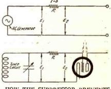
HOW THE SUPPRESSOR PREVENTS CURRENT FLOW
