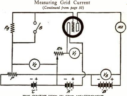
THE CIRCUIT USED IN GRID MEASUREMENT FIGURE 4: This schematic hook-up of the instruments used in the grid tests shows the simplicity and practicality of the new method.
