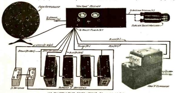
AN EXCELLENT OPERATING COMBINATION FIGURE 4: On account of its low current drain, "B" batteries may be employed quite economically with the New Home receiver. The socket antenna and "A" eliminator were also found very successful in this hook-up. SOLDERING COMES EASILY IF YOU KNOW THE RULES OF
