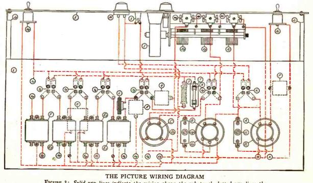
FIGURE 3: Solid RED lines indicate the wiring above the sub-panel, dotted RED lines the wiring beneath. The instruments are outlined in BLACK.
