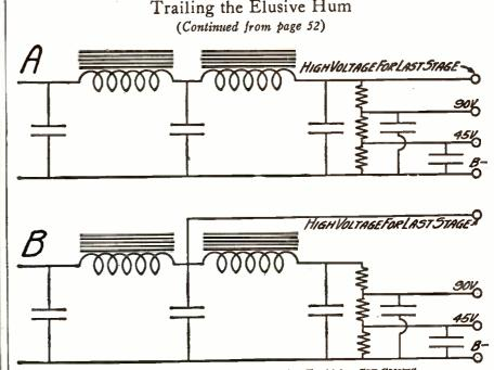
HOW TO RELIEVE OVERLOADED FILTER CIRCUITS FIGURE 3: At the top is a standard power-pack circuit with two chokes, filter condensers, and the usual voltage dividing resistances. Under a heavy load, such as occurs when a large power valve is used in the last stage, the inductance of the chokes may decrease so as to let an AC ripple through to the receiver. If the high voltage for the last valve is taken off through only one choke, as shown at B, this source of hum may be eliminated.
