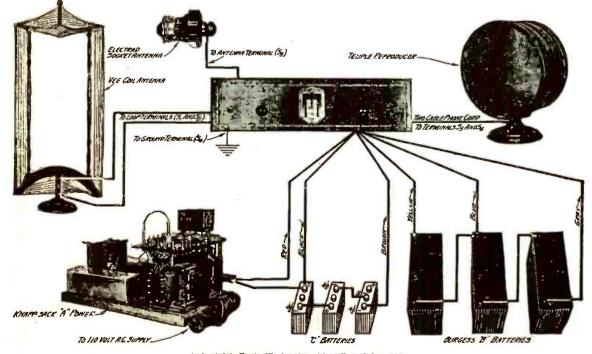
AN EFFICIENT OPERATING HOOK-UP FIGURE 4: The units illustrated here have been found by tests to give very good results when hooked up with the Victoreen as indicated by the heavy BLACK lines. Note that either a loop or socket antenna may be employed.
