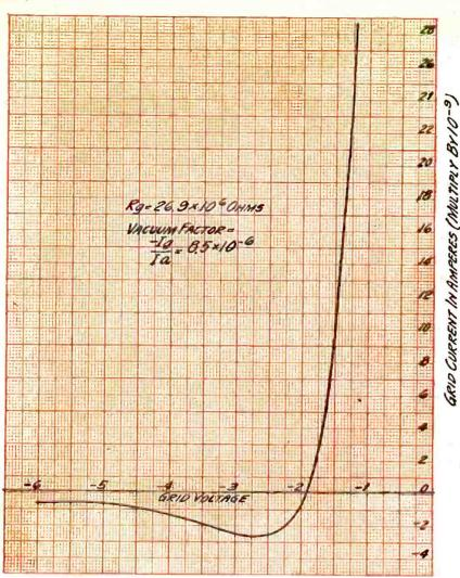
FIGURE 1: A grid-voltage, grid-current curve that shows the variation of these two factors in a vacuum valve.
