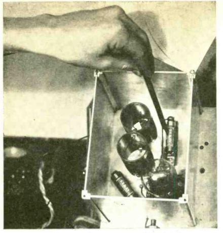
HOW GRID SUPPRESSORS ARE USED This picture shows one of the shielded stages of the LC-28 highfrequency amplifier, with the grid suppressor connected in the circuit between the tuning circuit and the grid of the valve.
