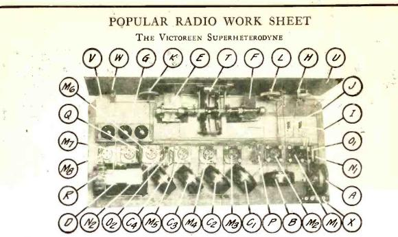
HOW THE INSTRUMENTS ARE MOUNTED FIGURE 1: The simplicity of the arrangement of the parts makes this superheterodyne an easy one for the novice to altempt.
