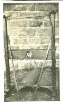
THE ROLL REPRODUCER READY FOR MOUNTING FIGURE 1: The two strips leaning on the frame are to be pressed into the grooves to keep the edges of the roll in position.
