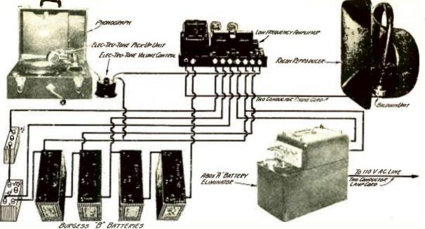
A COMPLETE PHONOGRAPH COMBINATION FIGURE 1: In this diagram the Rauland low-frequency amplifier, whose construction is described in the article below, is shown hooked up with a number of units into a combination that gives excellent results in reproduction from phonograph records.
