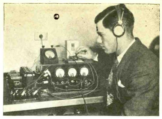
CHECKING THE PILOT FOR HUMS Among other tests at the POPULAR RADIO Laboratory, the Pilot power-pack was subjected to the test shown above, in which the unit was run under varying current loads, and the output tested for AC hum under these conditions.
