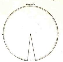
THE CUT-OUT OF THE FRONT CONE FIGURE 2: The wedge-shaped segment at the bottom of the diagram is cut out before the cementing process. The rest of the cutting is done after the cementing.
