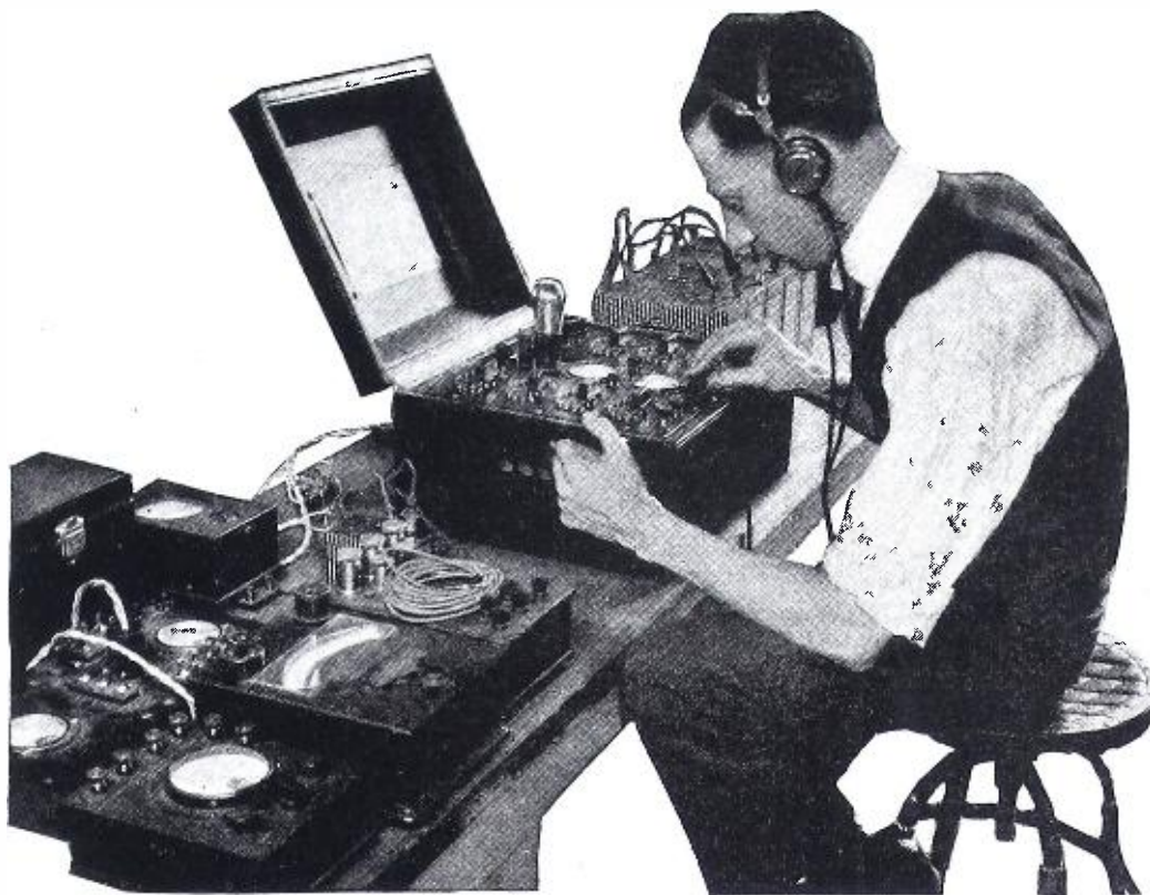
This photograph shows the marvelous Bridge Tube Tester in use in POPULAR RADIO Laboratory. No other instrument known provides such accurate or convenient means for charting tube characteristics. Only tubes successfully passing this and other severe tests may be advertised in POPULAR RADIO.
