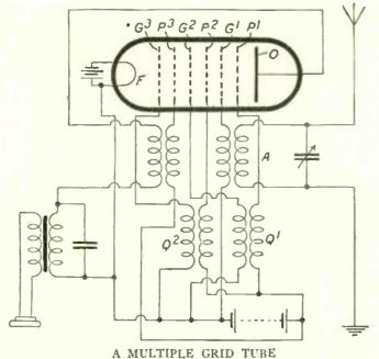
FIGURE 1: In this circuit, employing a special vacuum valve with six grids, a number of stages of high-frequency amplification are possible.
