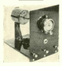
An Instrument That Will Automatically Turn a Radio Receiver "On" or "Off"
