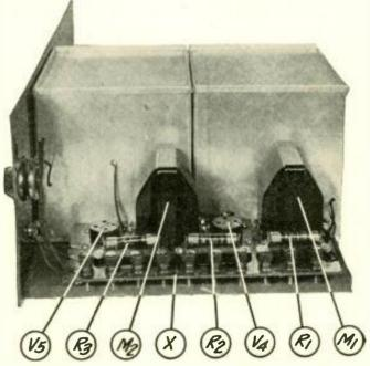
A VIEW OF THE SET FROM THE LOW-FREQUENCY END FIGURE 5: Here is shown the low-frequency amplifier in position at the side of the two box shields. The binding posts run along the edge.
