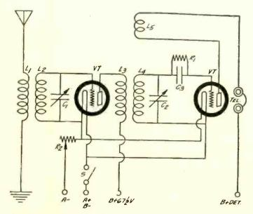
THE SCHEMATIC CIRCUIT FOR A SIMPLE TWO-TUBE SET This drawing gives the connections for one stage of high-frequency amplification with a regenerative detector It employs small valves that may easily be built up into a portable receiver.
