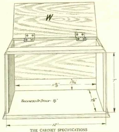
FIGURE 10: The cabinet used with the model of the Pre-selector is a standard stock size. For those who may wish to construct their own cabinets, however, the specifications are given here.
