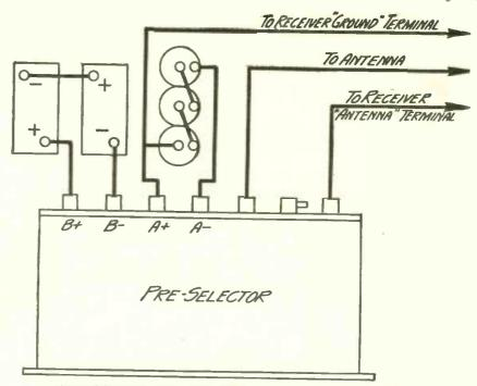
CONNECTIONS FOR THE USE OF SEPARATE BATTERIES
