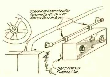
ONE WAY TO MOUNT A RECEIVER IN AN AUTOMOBILE Most five-passenger cars have a robe rail on the back of the front seat; it is a simple matter to install a receiving set on this rail, as indicated in the drawing above.
