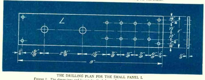
FIGURE 7: The dimensions and layout for the holes used in mounting the instruments and binding posts are clearly indicated. The sizes of the holes should be determined beforehand by measuring the sizes of the screws on the binding posts and the shafts of the two instruments that are to be mounted on this panel.
