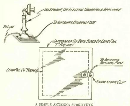
FIGURE 4: This diagram shows clearly a method for using the telephone line as an aerial where it is found impossible, on account of local conditions, to erect an outdoor antenna.
