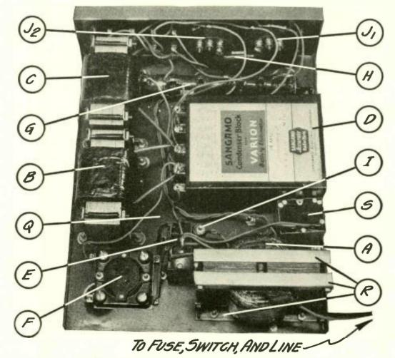
THE INNER ARRANGEMENT OF THE POWER-PACK
