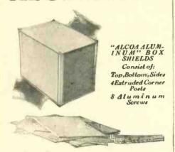
M EETING the highest radio standards—shipped to you in the most convenient knocked-down form for easy assembly. These Box Shields are made of heavy aluminum (080"—No. 12 B. & S.) and are supplied 5" x 9" x 6", which will cover most requirements. If the size does not meet your exact needs, change it—Aluminum is easy to work.
