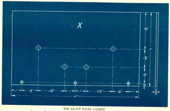
FIGURE 6: The panel should be laid out and drilled exactly as shown here. The diameter of the holes will depend on the size of the shafts and screws used. All the instruments employed are of the single hole mounting type.
