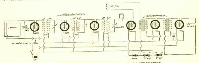
A GOOD CIRCUIT FOR A RECEIVER THAT IS USED IN AN AUTOMOBILE.
