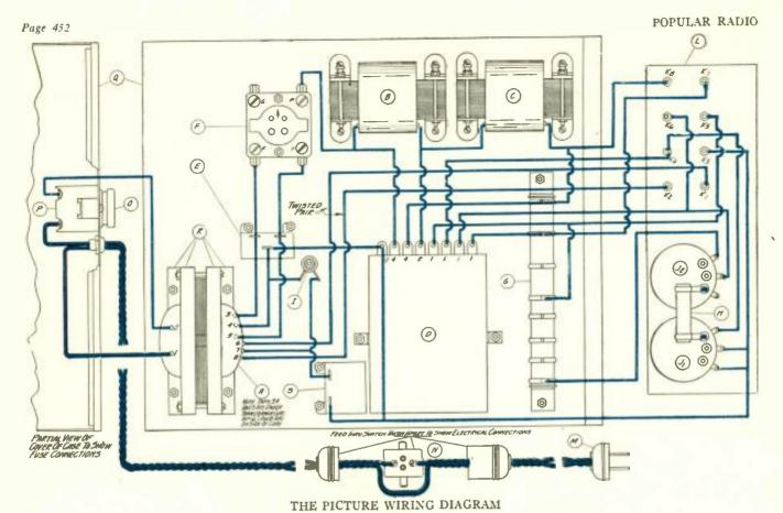
FIGURE 1: Here the wiring is shown in heavy Bluelines; the instruments themselves and the various parts and accessories are drawn in Black. The rectangle at the right shows the connections to be made on the binding post panel, the large middle rectangle those to the instruments mounted on the bottom half of the metal case. At the left is indicated the wiring of the instruments on the top half of the case.
