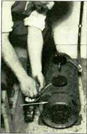
2: Dirty commutators on electric motors are a common source of interference.
