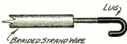
FIGURE 3: A little solder is allowed to run through the strands of wire to make the lug more permanent
