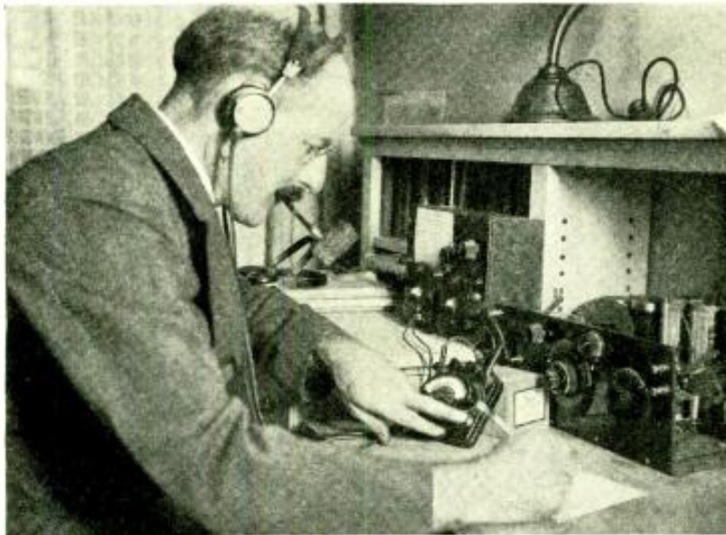
HERE IS A LABORATORY THAT ANY FAN CAN DUPLICATE With only the instruments shown above—a pair of headphones, a simple receiving set and just one meter—the author made all of the experiments that are described in this article.
