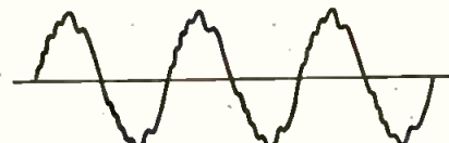
WAVESHAPE OF A VIOLIN - SIX HARMONICS
